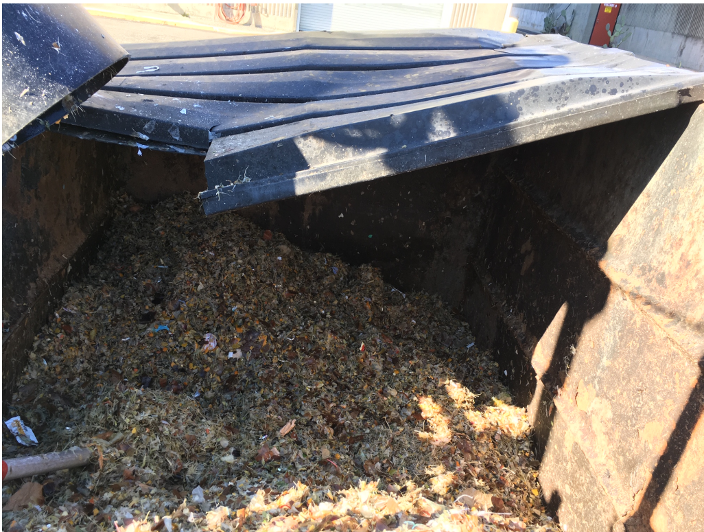
Figure 5.3 CMSA Contaminants Removed by Paddle Finisher
