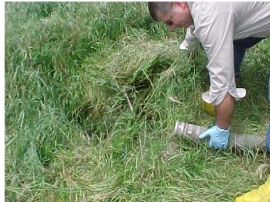
Photo 16. End of flexible hose from which septic was discharged (note erosion pothole at pipe outlet)
