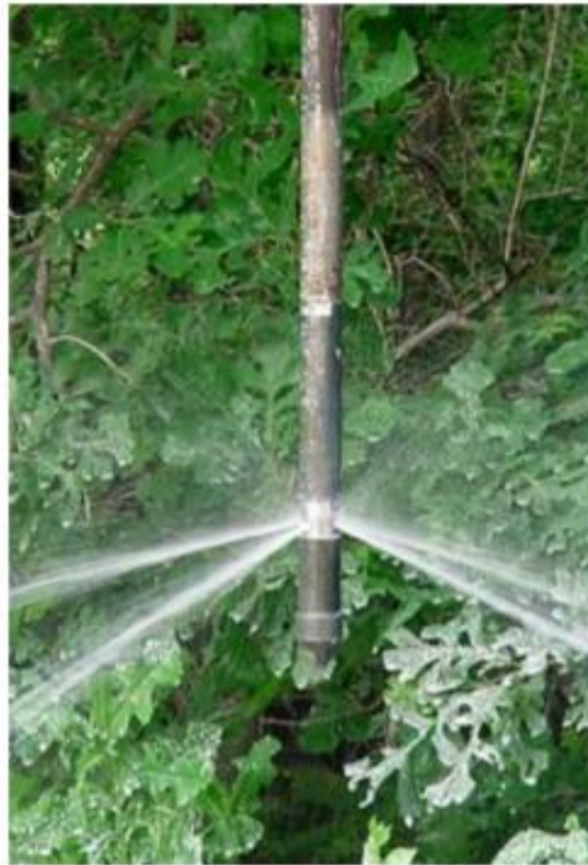
PRESSURE ACTIVATED INJECTION TOOL PROBE SHOWING FLUID INJECTION PATTERN/ORIENTATION
