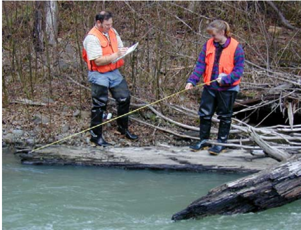
Photograph 7. Measuring large woody debris volume.
