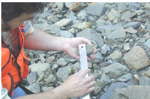
Photograph 5. Measuring particle size of the streambed surface.
