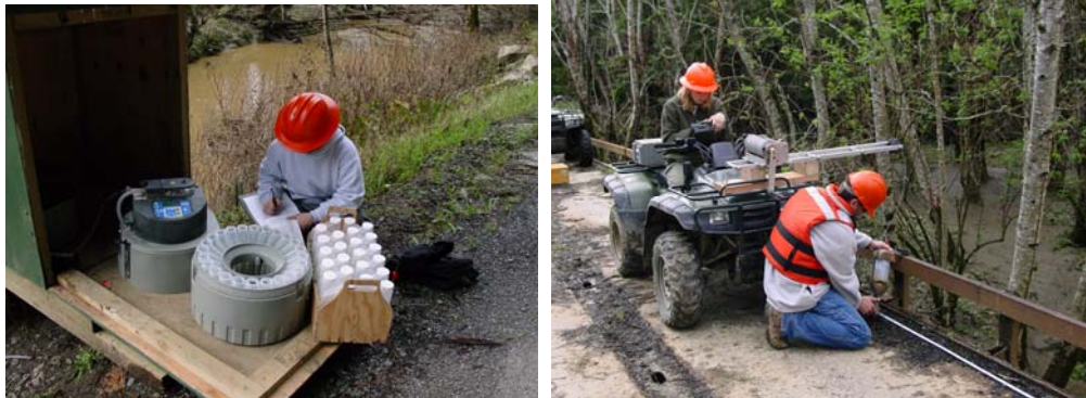
Photograph 3. Turbidity and stream flow field sampling.
