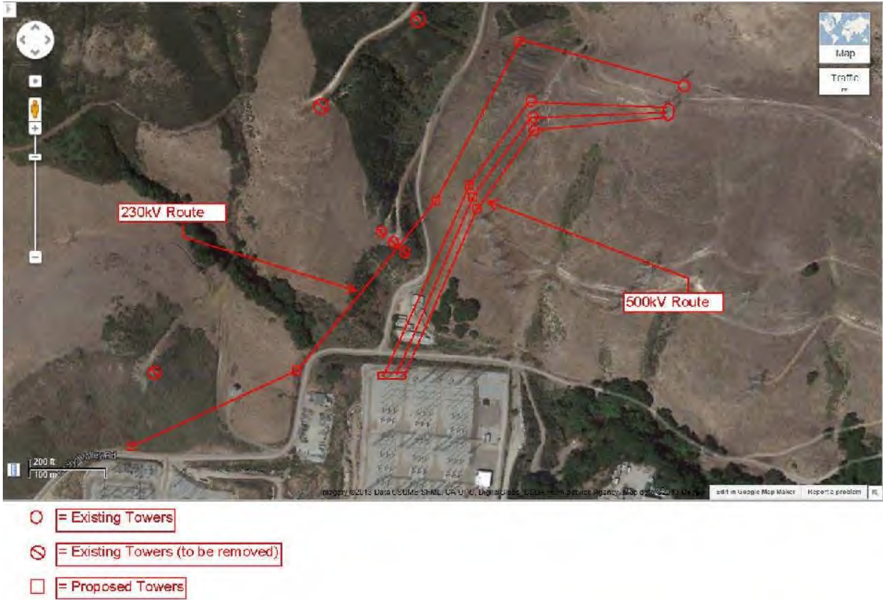
Figure 4.3-6. Existing 230 kV and 500 kV Power Line Rerouting
