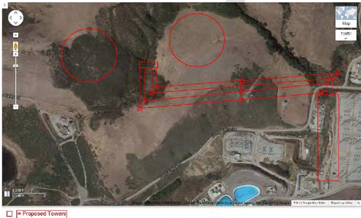
Figure 4.3-7. 500 kV Power Supply to the Cooling Towers
