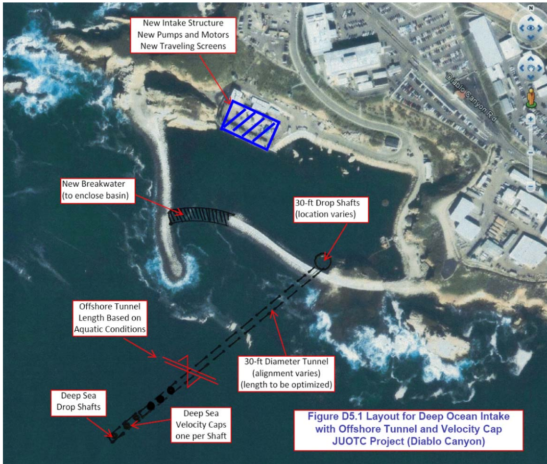
Figure DW-1. Layout for Deep Ocean Intake with Offshore Tunnel and Velocity Cap
