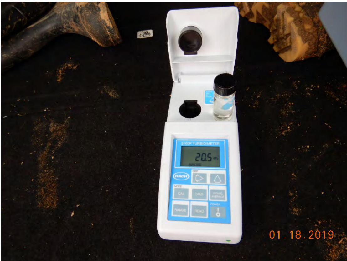
Photo 12. Turbidity of water sample collected upstream of Project's dewatering activities.
