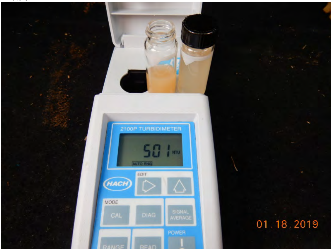
Photo 6. Turbidity of discharges. A diluted sample comprised of 25% discharge sample and 75% drinking water had a turbidity of 501 NTU. The diluted sample shown on meter with a cap. The un-diluted discharge sample shown on the meter without a cap.
