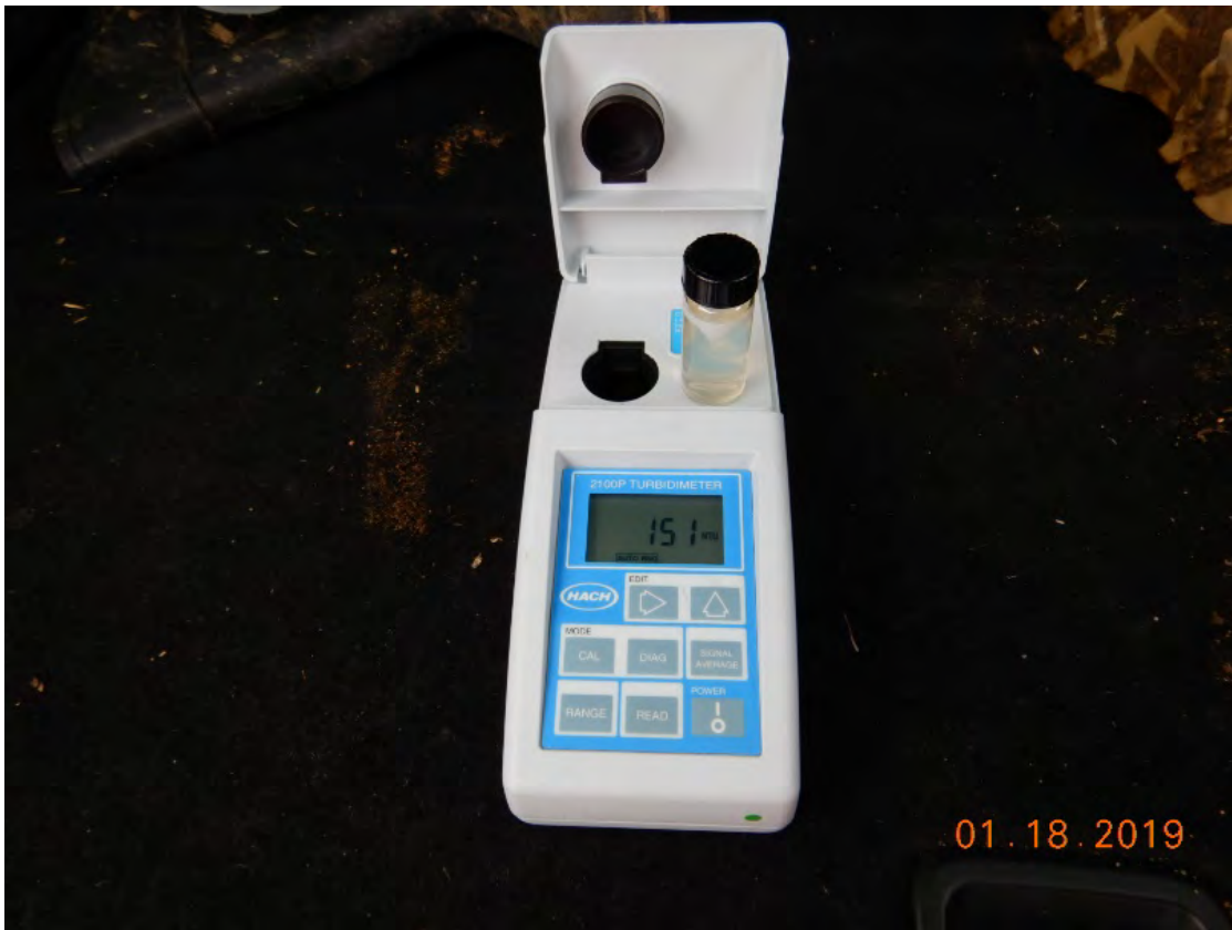
Photo 10. Turbidity of water in Secret Ravine tributary downstream from Project's dewatering activities.
