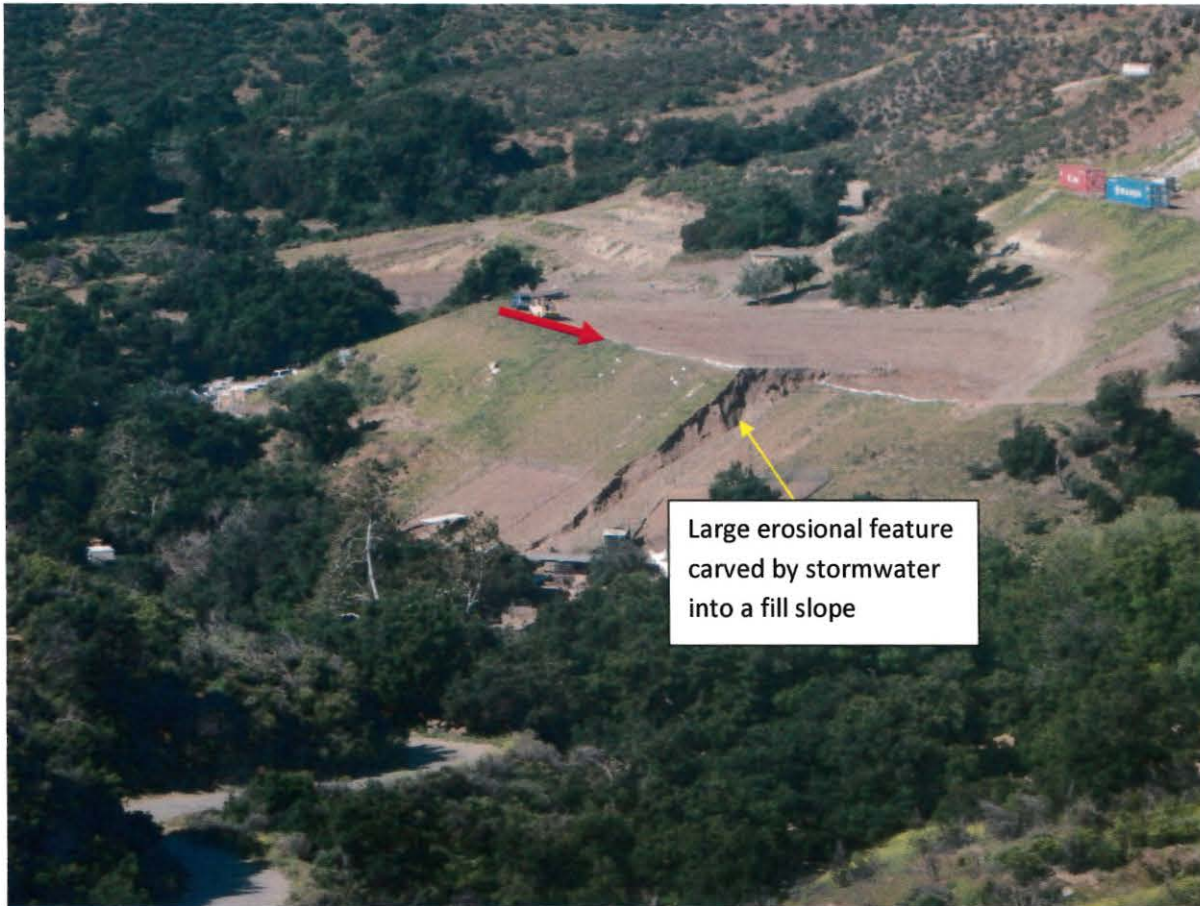
Photo 3. View looking southwest from Photo Location 1. Showing canyon carved into slope in parcels 2821-009-030 and 2821-009-031, which are owned by Mr. Wayne Fishback and Cepheid V, LLC respectively. The base elevation of the large erosional scour is in the immediate vicinity of the Ybarra Creek bed. It can be inferred from this photo that all the stormwater scoured fill materials were transported into Ybarra Creek. The red arrow indicates the remnant sandbag wall, presumably the wall that Mr. Fishback alleges was sabotaged. The photo was taken at Longitude -118 36 21.75 and Latitude 34 18 22.79 on April 12, 2017.
