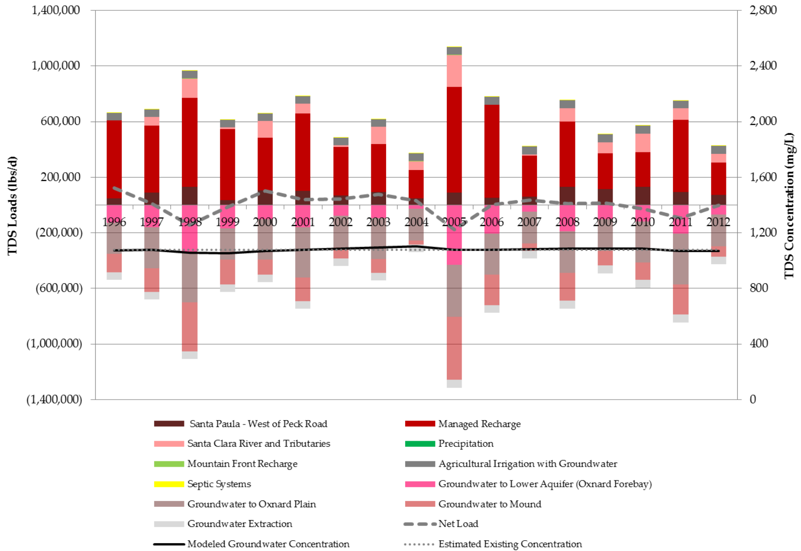
Figure 7-34 Modeled Annual TDS Loads and Concentrations in Groundwater for Oxnard Forebay Basin
