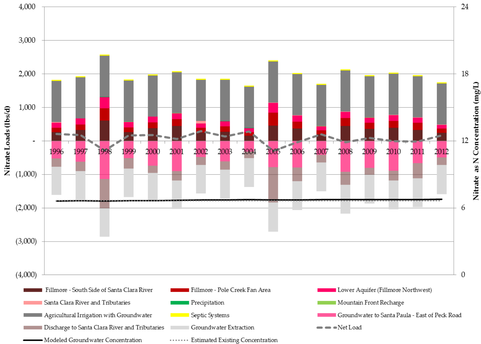
Figure 7-24 Modeled Annual Nitrate-N Loads and Concentrations in Groundwater for Fillmore Basin – Remaining Area
