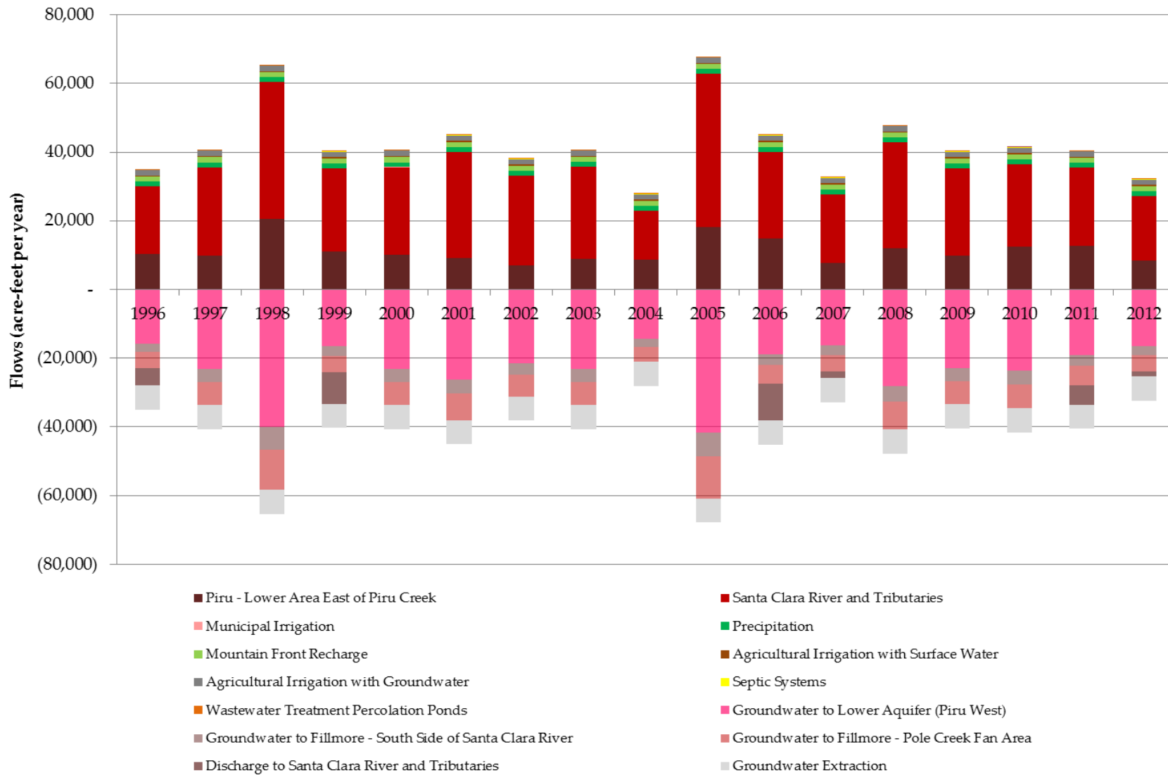
Figure 7-9 Modeled Annual Inflows and Outflows for Piru Basin – Lower Area West of Piru Creek
