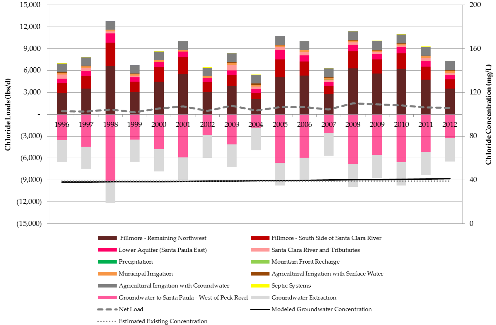
Figure 7-27 Modeled Annual Chloride Loads and Concentrations in Groundwater for Santa Paula Basin – East of Peck Road Area
