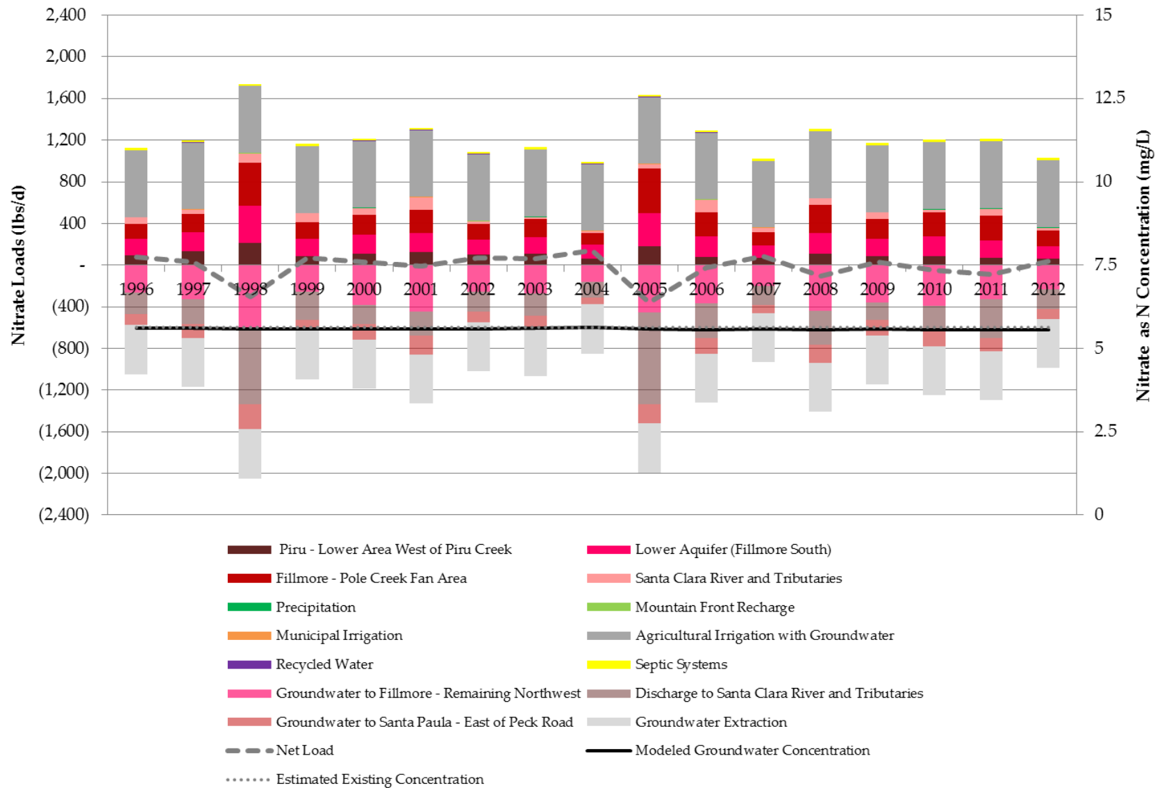
Figure 7-20 Modeled Annual Nitrate-N Loads and Concentrations in Groundwater for Fillmore Basin – South of Santa Clara River
