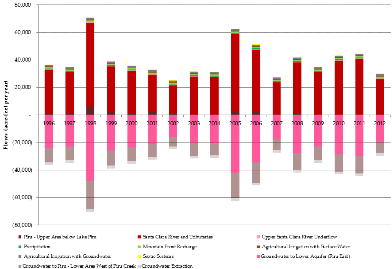
Figure 7-5 Modeled Annual Inflows and Outflows for Piru Basin – Lower Area East of Piru Creek
