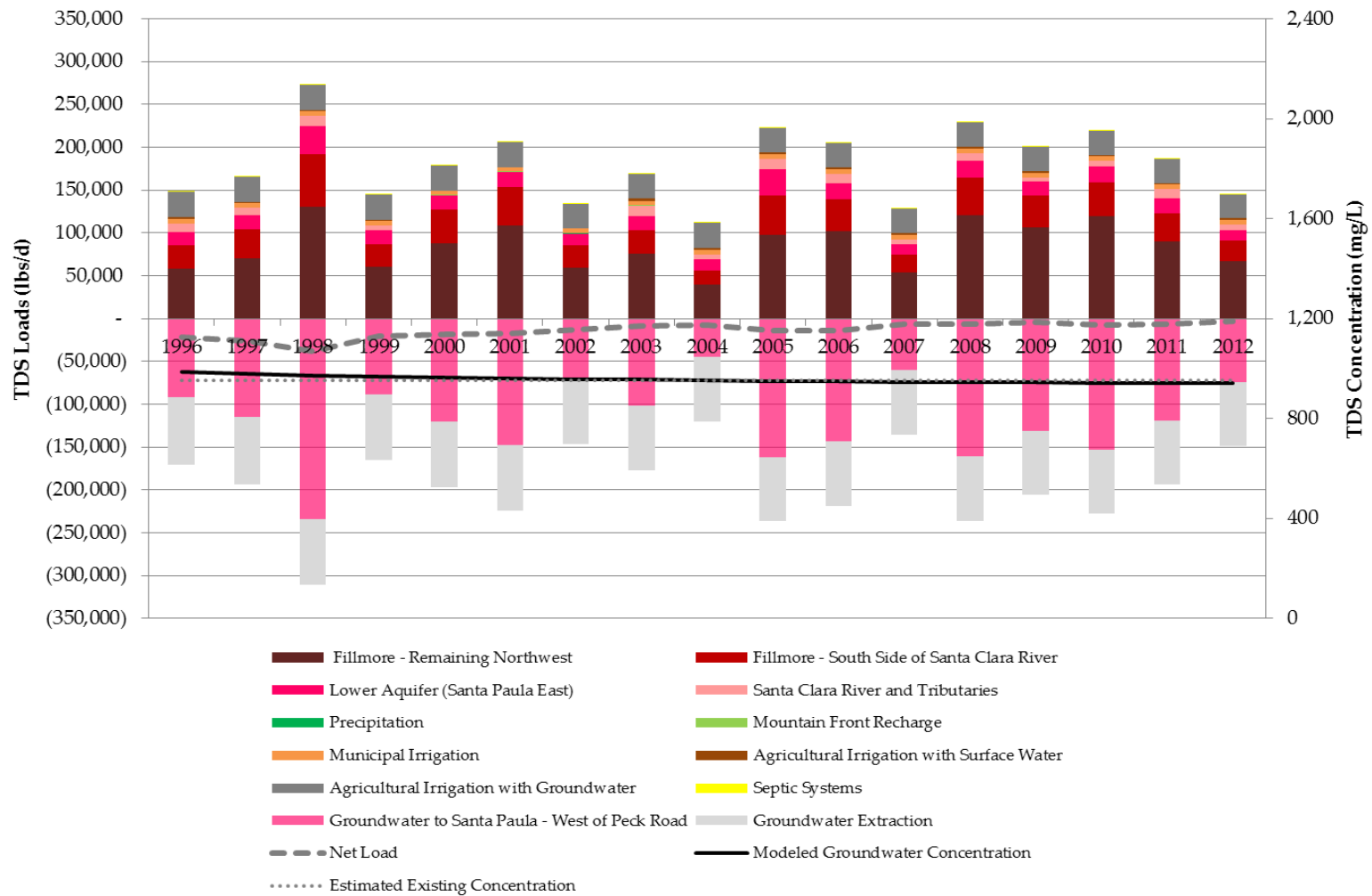
Figure 7-26 Modeled Annual TDS Loads and Concentrations in Groundwater for Santa Paula Basin – East of Peck Road
