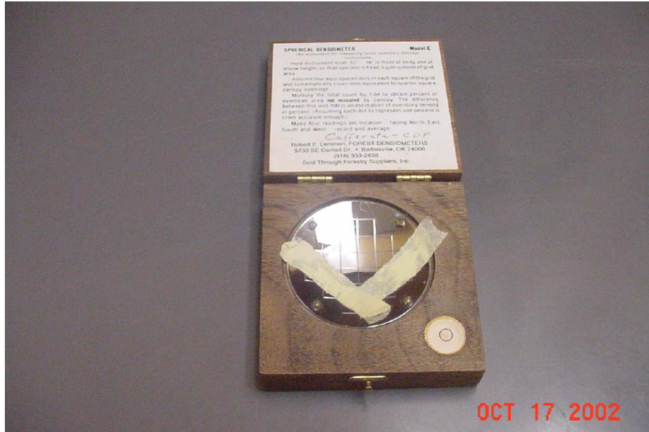
Figure 5. Concave spherical densiometer used for canopy measurements from 1996 to 1998 (the Strickler (1959) modification was utilized in 1997 and 1998 to reduce bias).
