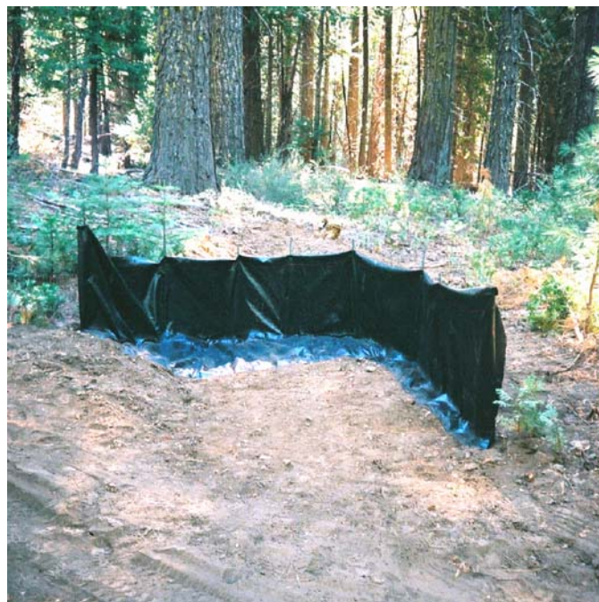
Figure 1. Example of one of 147 sediment fences installed to measure sediment production rates in the central Sierra Nevada Mountains (photo by Drew Coe used with permission).
