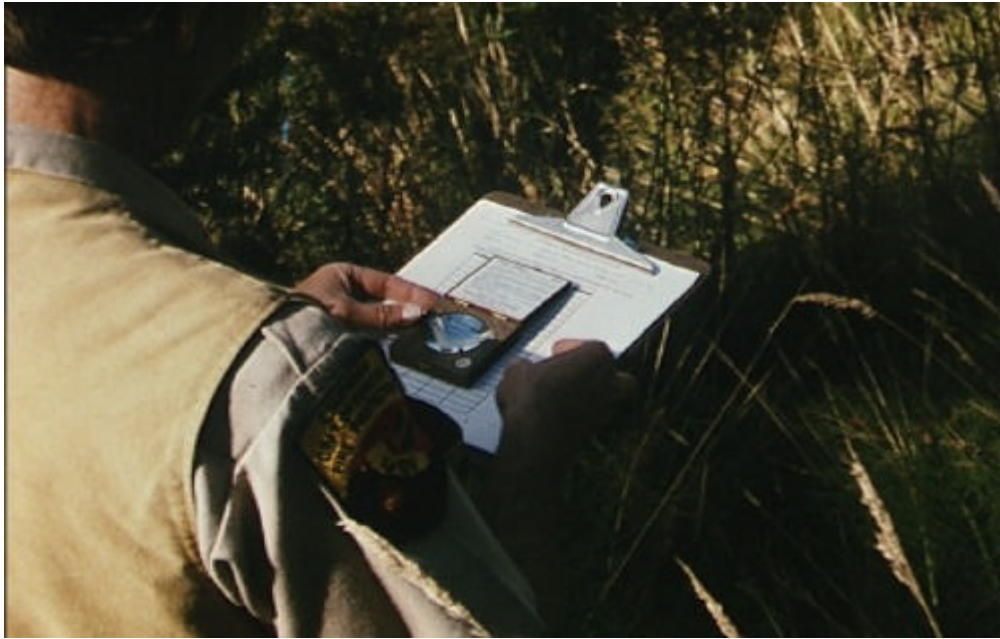
Figure 2. Concave spherical densiometer with the Strickler (1959) modification.
