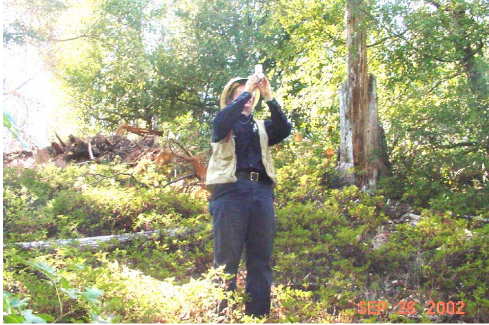
Figure 7. The sighting tube in use in the field. This instrument was utilized for obtaining an unbiased estimate of canopy cover from 1999 through 2001.
