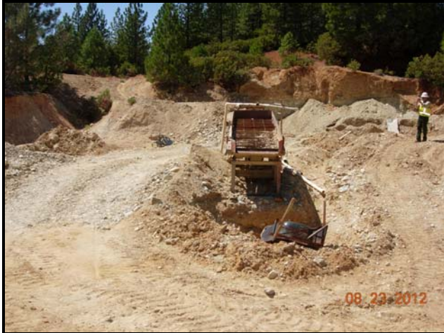
Photo 13. Shows a small wash plant used for screening and washing of mined material.
