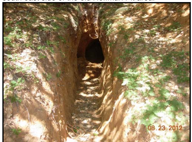
Photo 18. Backhoe trench leading to a small underground mine working between Hoffman Pit and the Britt Mine.
