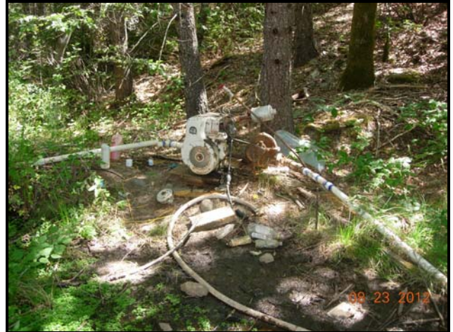
Photo 22. Water pump at the Britt Mine presumably used to pump water to the Hoffman Pit mining operation.
