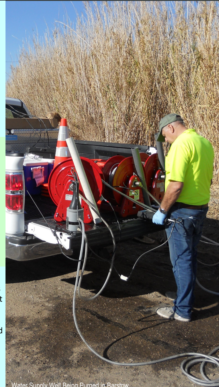
Water Supply Well Being Purged in Barstow. Courtesy of the Lahontan Regional Water Board
