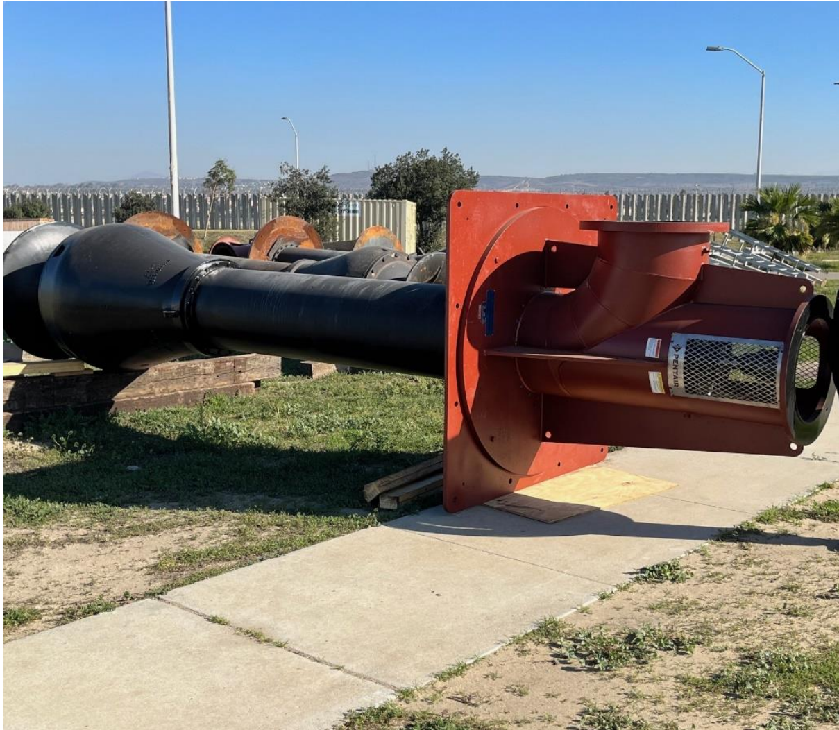
Figure 4: Closer view of one of the new influent pumps. (USIBWC 12/13/2023)
