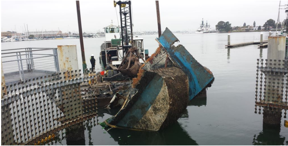
Photo 1. Derelict vessel being lifted onto a barge by crane at the "reflecting pier" at Union Point Park in Oakland (Courtesy CalRecycle staff).
