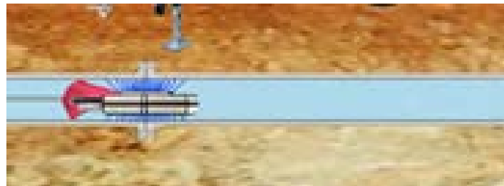
Inline leak detection
