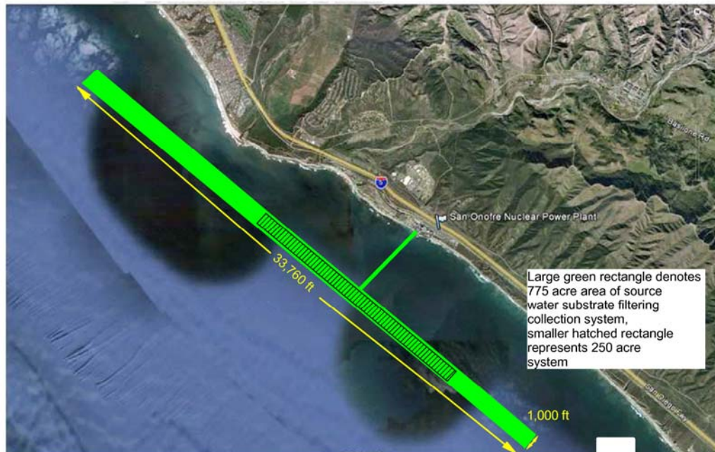
Figure SWS-6. Conceptual Layout of Source Water Substrate Filtering Collection System at SONGS
