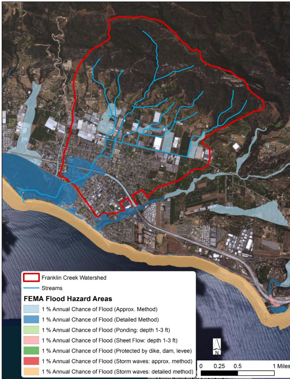
Figure 13. Flood hazard areas within the Franklin Creek watershed (FEMA, 2015).
