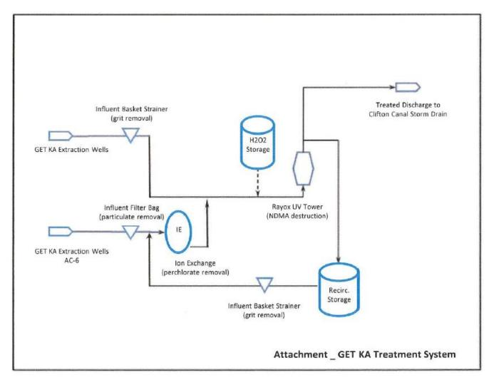
13. **ATTACHMENT C – FLOW SCHEMATICS.** Replace Attachment C-10. Miscellaneous Treatment Systems with the figure shown below.
