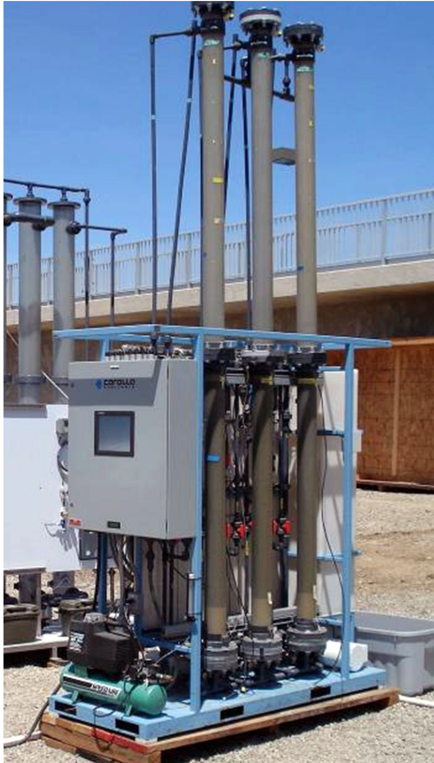
Figure 6 BAF PILOT SKID SET UP ON SITE AT BOLLMAN WTP CALIFORNIA DEPARTMENT OF WATER RESOURCES CALIFORNIA DEPARTMENT OF PUBLIC HEALTH
