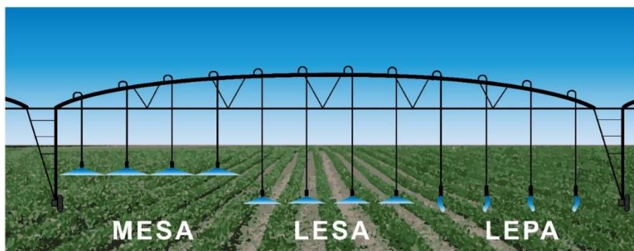
Figure 16. Types of pivot irrigation methods. Mid-elevation spray application (MESA) uses a pivot system where nozzles are spaced about 7.5 feet to 20 feet apart, 3 feet to 6 feet above the ground, and have a wetting diameter of 20 feet to 75 feet. Water is delivered above the crop canopy. MESA has 78 percent water efficiency. Low elevation spray application (LESA) uses a pivot system where nozzles are 4.5 feet to 5 feet apart, 1 foot to 3.5 feet above the ground, and have a wetting diameter of 12 feet to 30 feet. LESA has 88 percent water efficiency. Low energy precision application (LEPA) uses a pivot system with sprinklers or bubblers that are spaced 2.5 feet to 3.5 feet apart and are about 1 foot to 2 feet above the ground. LEPA has 95 percent water efficiency (Holt et al., 2021). Image source: Bayer (2019).
