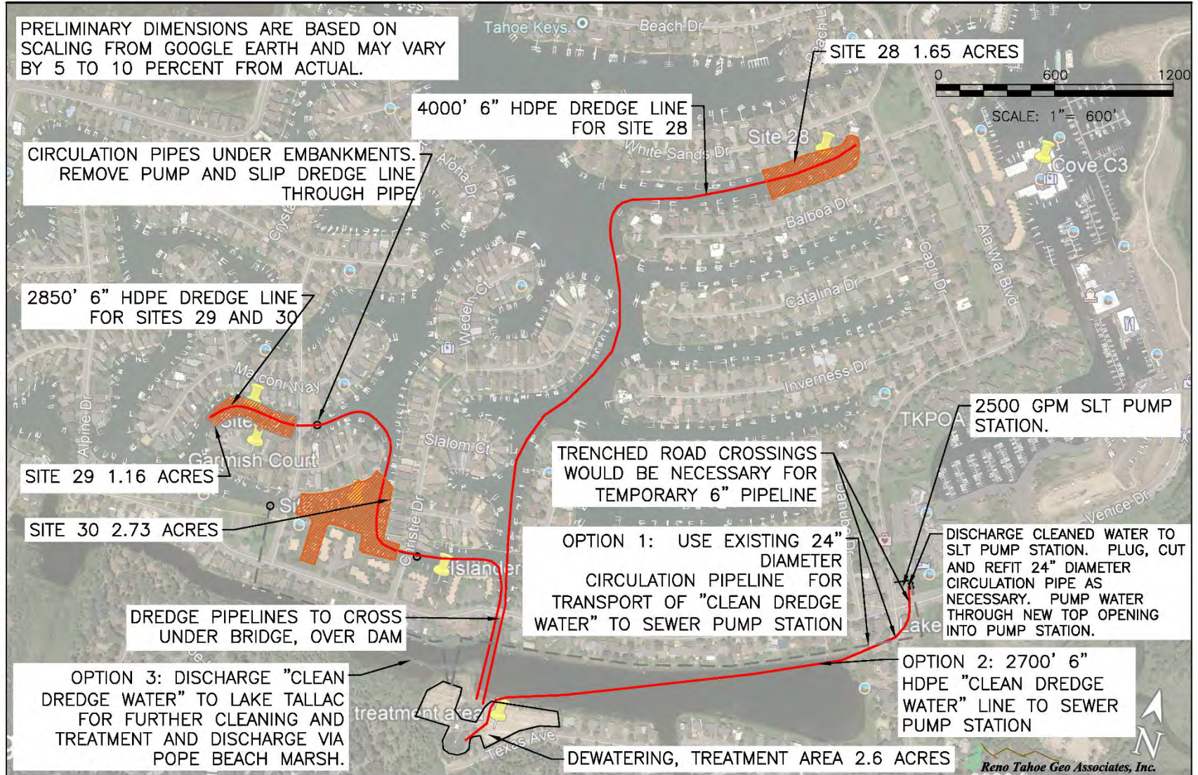
Figure 2-10 Preliminary Layout of Suction Dredging Operations.
