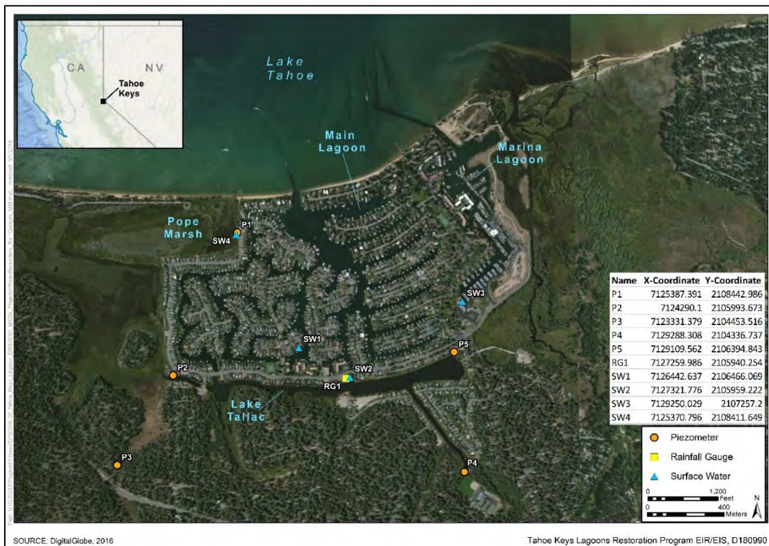
Figure 1. Locations and coordinates for piezometers, surface water level recorders, and a rain gauge at Tahoe Keys.
