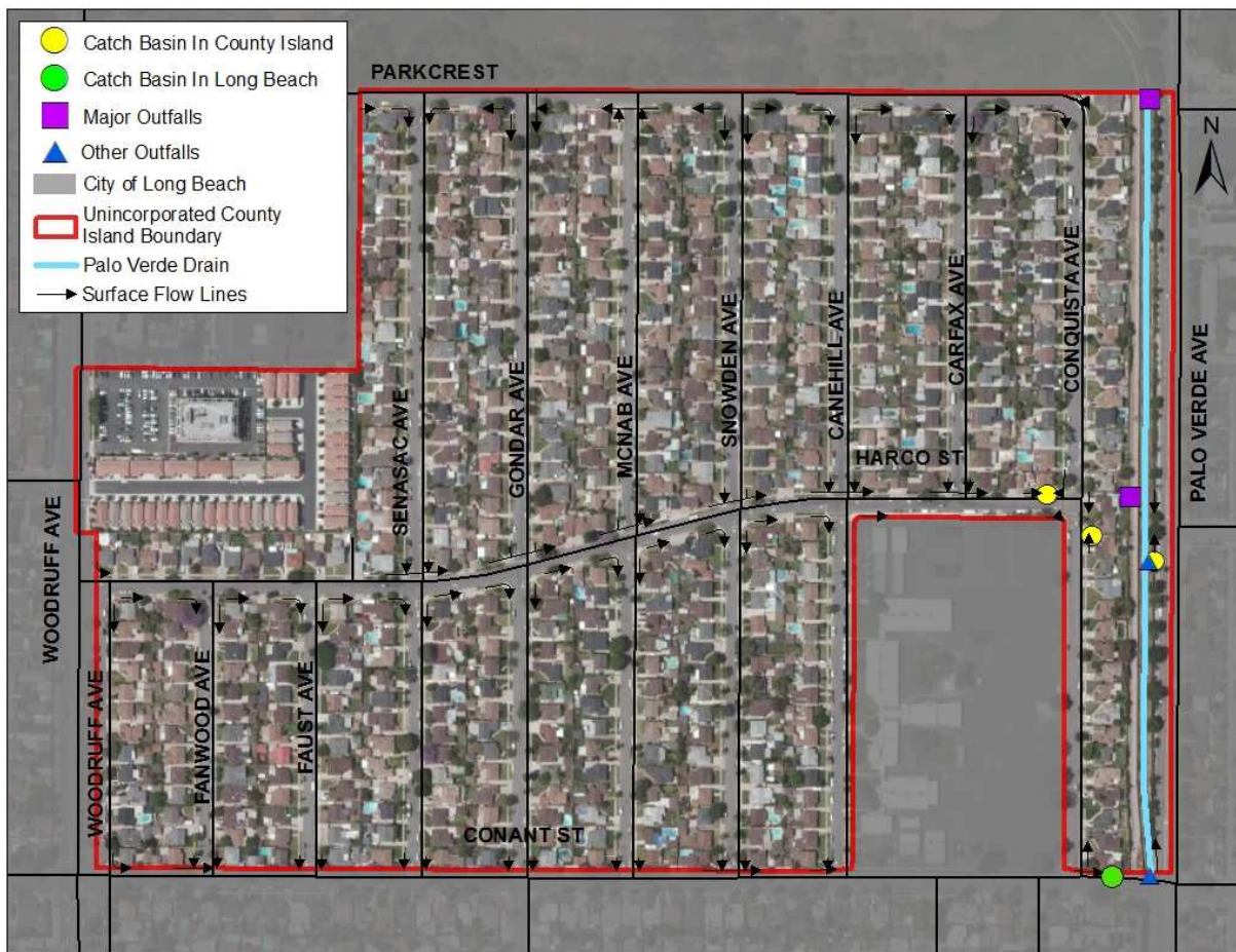
Figure 14: MS4 Outfalls and Flow Direction in County Island
