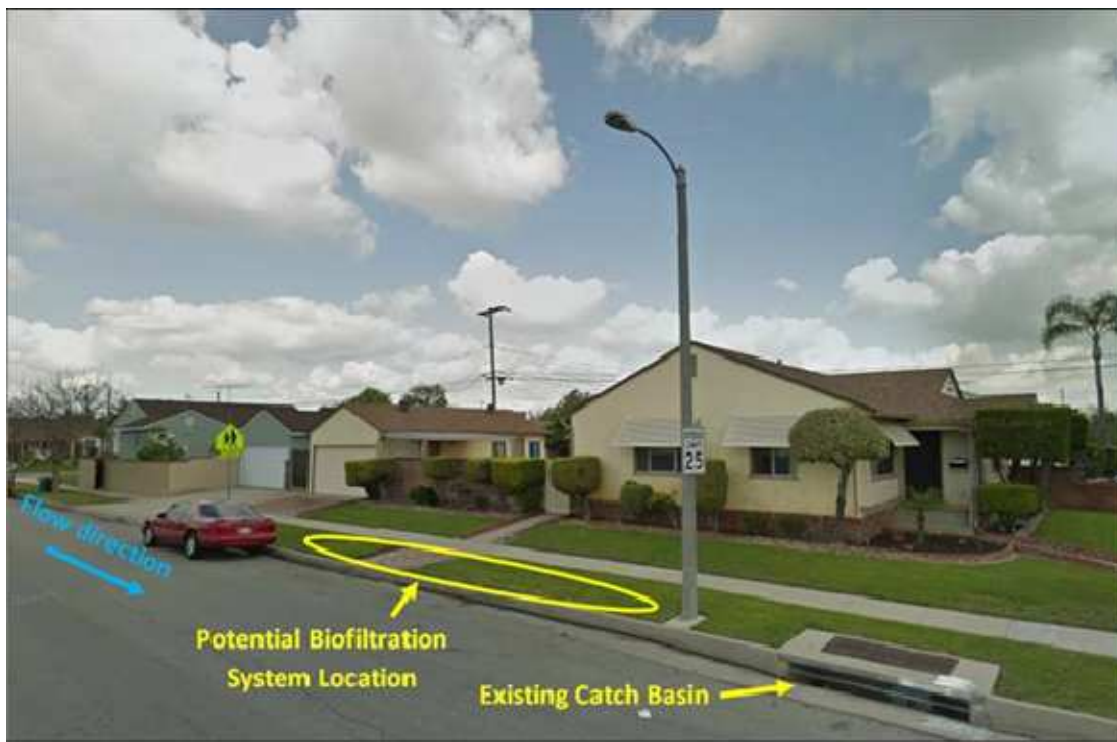
Figure 13: Potential Biofiltration System Location
