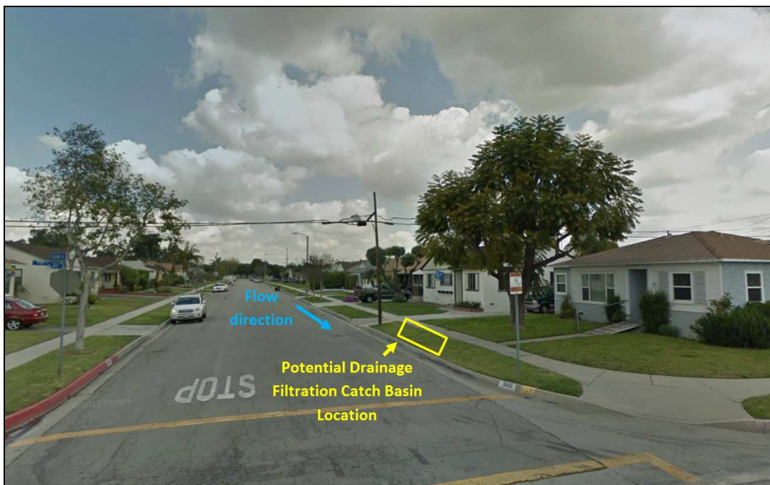
Figure 15: Potential Drainage Filtration Catch Basin Locations
