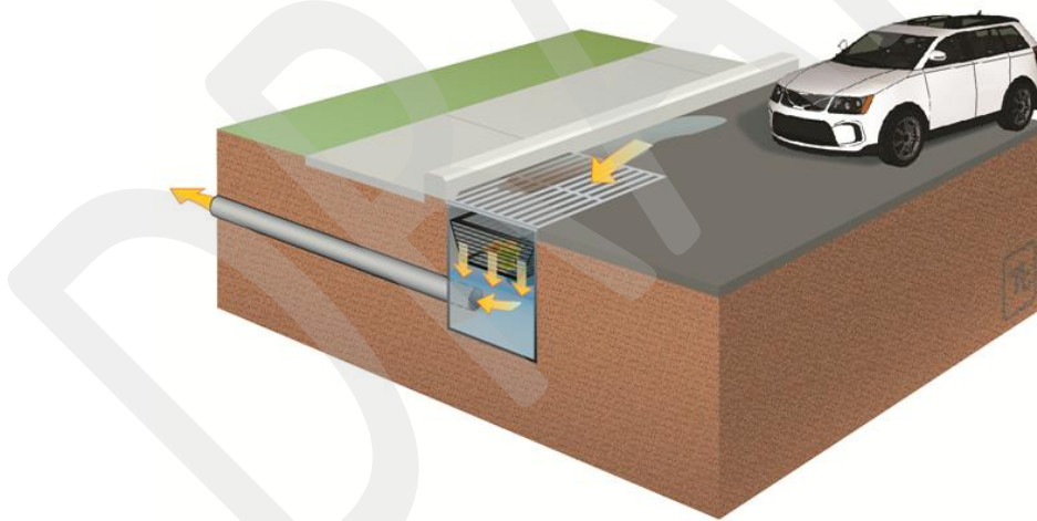
Figure 3-12: Pre-treatment BMP schematic
