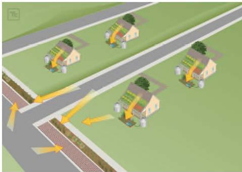
Figure 3-1: Distributed BMP Schematic
