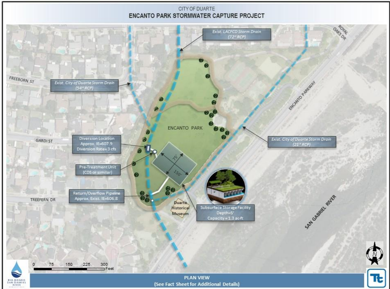
Figure 8. Encanto Park Stormwater Capture Project Site Layout
