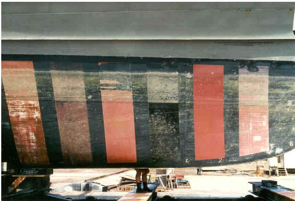
Figure 13: Starboard side strips on HMAS BENDIGO, April 1998
