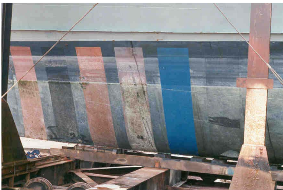
Figure 14: Port side strips on HMAS BUNBURY, February 1996. Blue strip is Ecoloflex
