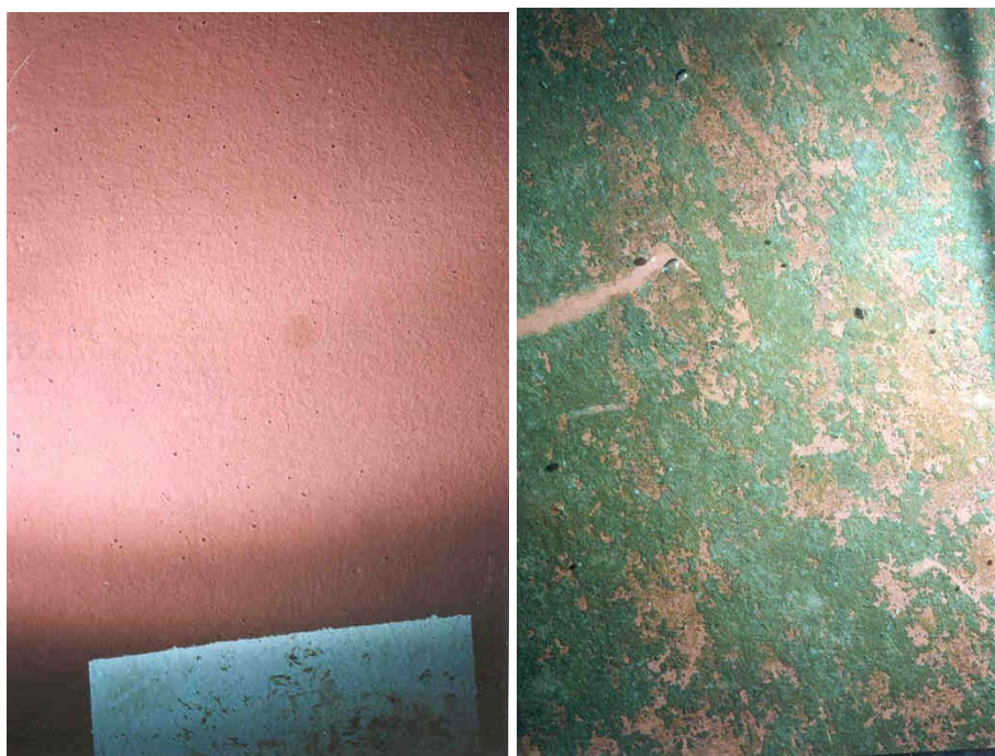
Figure 10: Underwater photographs of Ecoloflex strip on HMAS BENDIGO in January 1995 (left) and October 1997 (right) showing slime
