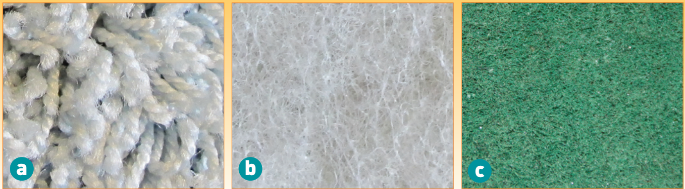
Examples of common hull cleaning tools: (a) carpet, (b) white pad, and (c) green pad
