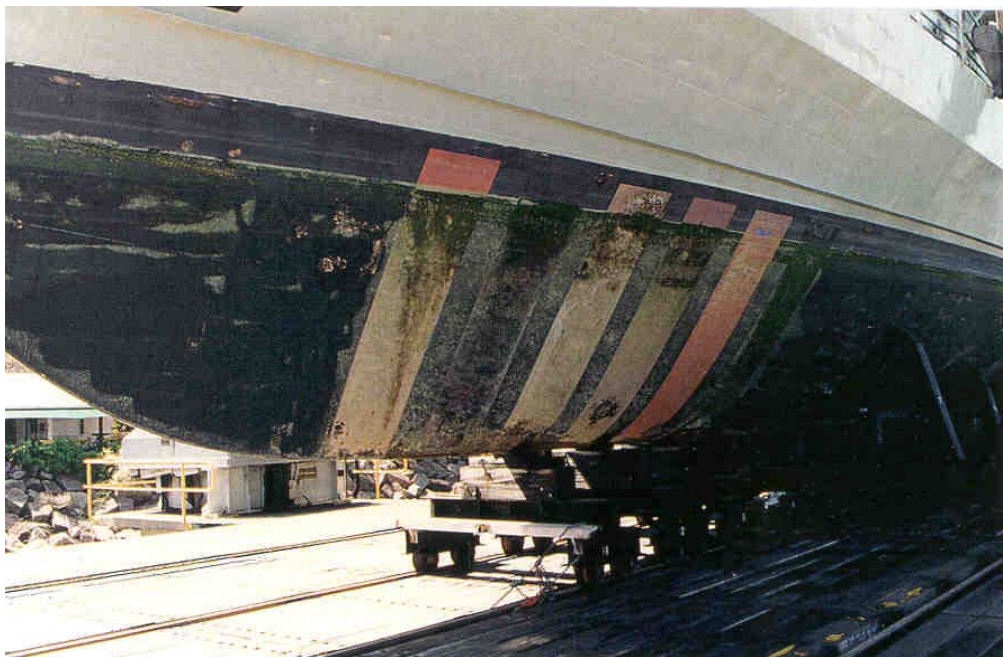
Figure 16: Port side strips on HMAS BUNBURY, May 1998
