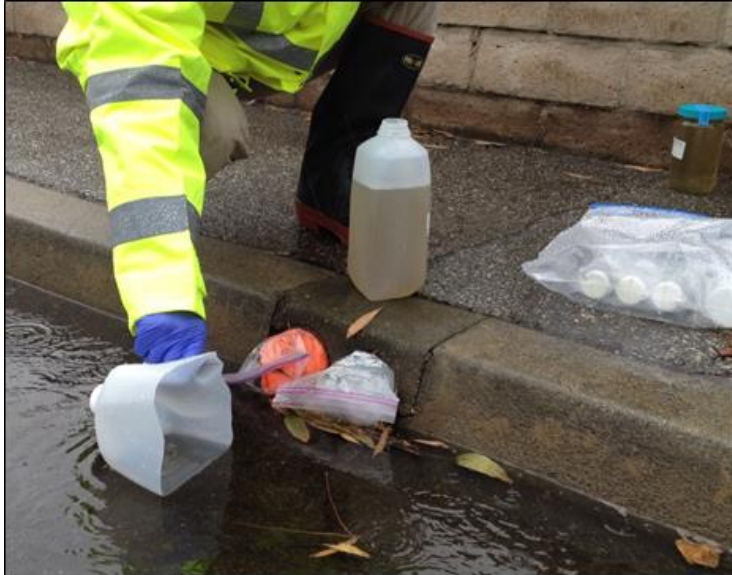
Figure 2-10 Typical Parking Lot 7 site with drains plugged and sample collected by scoop
