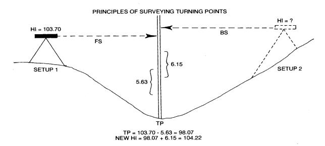
Figure 8. Using *turning points* to move the instrument.
