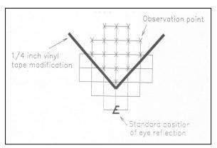
Figure D-1: Modified grid of spherical densiometer.
