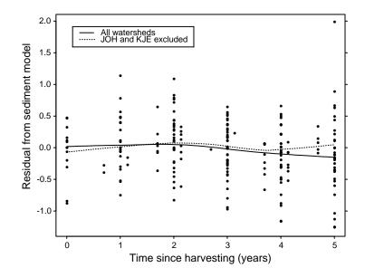
Figure 23. Relation between residuals from sediment model {(24),(17),(18)} and time after logging. Curves are fit by loess method [Cleveland, 1979], with and without the anomalous watersheds JOH and KJE.
