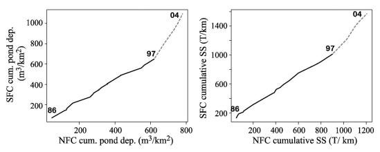
Figure 2. Double mass curve of South Fork pond accumulations and suspended sediment relative to North Fork 1986 through 2004.
