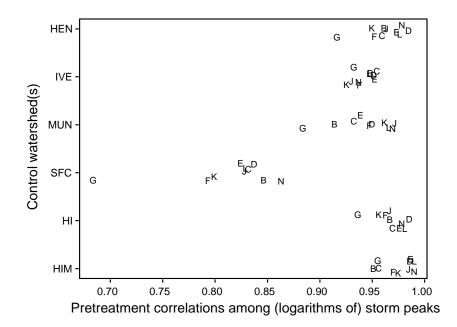
Figure 3. Pretreatment correlations between logarithms of storm peak at treated watersheds and alternative control watersheds. Letters designate watersheds (e.g. G is watershed GIB). Random noise has been added to the vertical plotting positions to improve readability.
