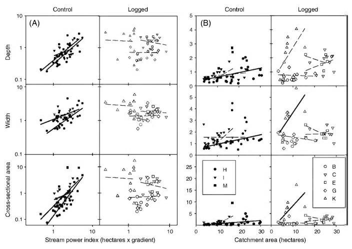
Fig. 5. Variation in mean segment depth (m), width (m), and cross-sectional area (m<sup>2</sup>) with (A) stream power index and (B) catchment area in control and logged tributaries of North Fork Caspar Creek. Relations significant at the 0.05 level are depicted by solid lines.
