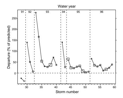
Figure 5. Post-logging departures of storm peaks (as percentage of predicted) at watershed EAG from those predicted from pretreatment regression on HI control. Axes are logarithmic. Symbol sizes indicate relative size of storm peak at HI control. Vertical dotted lines separate water years. About half the watershed was winter-logged before storm 28 and logging was completed by storm 30.
