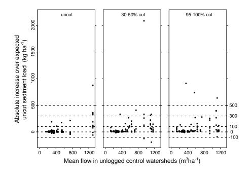
Figure 27. Absolute increase over expected uncut storm sediment load as related to mean of storm runoff volume in HIM control watersheds for uncut (before treatment), partly (30-50%) clear-cut, and (95-100%) clear-cut watersheds. Bias-corrected predictions are from model {(25),(17),(18)} with disturbance set to zero.
