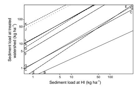
Figure 22. Regression lines for each watershed based on intercepts  $b_{0i}$  and slopes  $b_{1i}$  of sediment model {(24),(17),(18)}, with  $\beta_6$  fixed at zero. Letters designate watersheds (e.g. G is watershed GIB).
