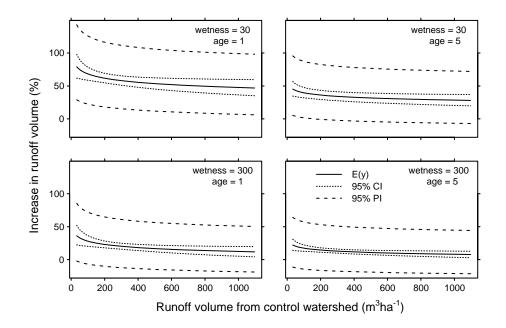
Figure 15. The effect of wetness and age after cutting on predictions from storm runoff volume model {(10),(17),(18)}, after clear-cutting 50% of a 20 ha watershed. Expected increases and 95% confidence (CI) and prediction (PI) intervals are shown for two levels of antecedent wetness 1 and 5 years after cutting.
