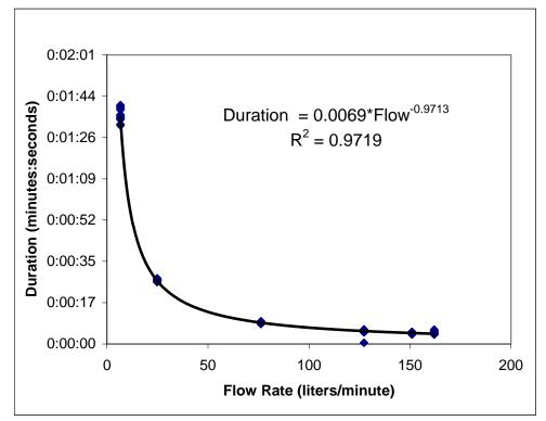
**Fig. 2: Pre-season calibration curve for site 10.** Fitting a power curve to tipping time data at known flow rates provides a relation between tipping times, downloaded from the data logger, and flow rates. After this relation is inverted to express flow as a function of duration, it is used in equation 1 below to estimate total runoff.
