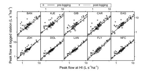
Figure 4. Relation between peak streamflow in the 10 treated tributaries in the North Fork of Caspar Creek, and that of the HI control. Post-logging relations were fitted by locally weighted regression [Cleveland, 1979]. The top row represents 95-100% clear-cut watersheds.
