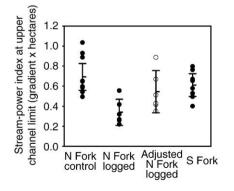
**Fig. 7.** Distribution of stream power indices at the upper limits of tributary channels. Error bars indicate the 95% confidence interval around the means (horizontal lines). "Adjusted" values account for hydrologic change after North Fork logging (see text Section 5.3.1).
