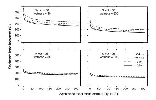
Figure 20. Effect of watershed area on predictions from sediment model {(24),(17),(18)} for two levels of cutting and two levels of antecedent wetness. Watershed areas are those of ARF, FLY, DOL, and BAN (Table 1). Predictions are for first year after cutting with  $x_{ij}^{(1)} = x_{ij}^{(2)} = 12 \text{ m ha}^{-1}$ .
