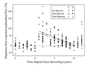
**Figure 5**—Storm flow volumes observed in North Fork clear-cut units C and E from HY1986 through HY2003. Expected undisturbed flow is based on log-log regressions of pre-harvest flows at CAR and EAG on the mean of the corresponding storm flows at control watersheds HEN and IVE.
