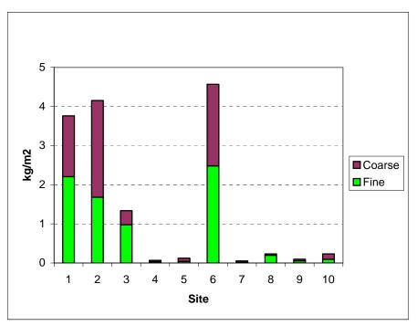
**Fig. 3: Coarse and Fine Sediment Production, HY2005-2006.** Data are normalized by area. Sites 1-6 are unsurfaced while sites 7–10 are rocked. While the highest-producing road segments were all unsurfaced, two unsurfaced segments (4 and 5) produced less sediment than the higher-producing rocked segments (8 and 10).
