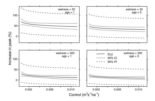
Figure 14. The effect of wetness and age after cutting on predictions from storm peak model {(10), (16),(18)} after clear-cutting 50% of a 20 ha watershed. Expected increases and 95% confidence (CI) and prediction (PI) intervals are shown for two levels of antecedent wetness 1 and 5 years after cutting.
