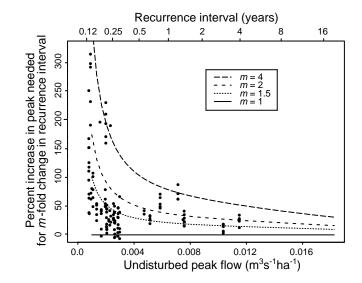
Figure 29. The curve shows the percentage increase in peak flow necessary to reach a size that formerly had 1 to 4 times the recurrence interval. The data points are from Figure 13 (third frame), representing the observed percentage increases in storm peak flow (based on the HI control, plotted on the abscissa) in 95-100% clear-cut watersheds.
