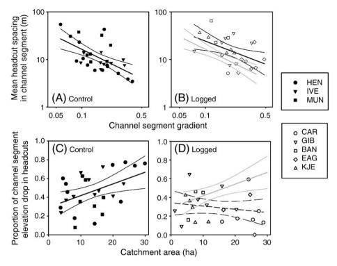
**Fig. 4.** Headcut spacing as a function of channel gradient in 50-m reaches of North Fork (A) control ( $r^2 = 0.36$ ) and (B) logged ( $r^2 = 0.23$ ) tributaries; and relative importance of elevation drop from headcuts in (C) control ( $r^2 = 0.20$ ) and (D) logged ( $r^2 = 0.03$ ) tributaries of North Fork Caspar Creek. The gray lines in Fig. 4B and D depict the regression and 95% confidence band for controls. Dashed lines indicate relations not significant at the 0.05 level.
