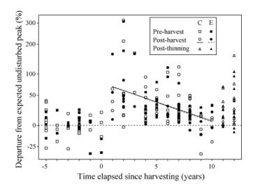
**Figure 2**—Peak flows observed in North Fork clear-cut units C and E from HY1986 through HY2003. Expected undisturbed peak is based on log-log regressions of preharvest peak flows at CAR and EAG on the mean of the corresponding peak flows at control watersheds HEN and IVE.
