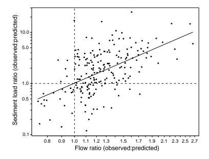
Figure 18. Relation between post-treatment sediment load departures from pretreatment relationship (3) and flow departures  $\Delta q_{ij}^{(1)}$ . Departures are expressed as the ratio of observed to predicted response.
