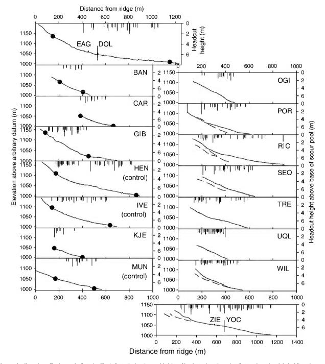
Fig. 3. Surveyed valley-axis profiles in gaged tributaries. Tics indicate the locations and heights of headcuts along the main tributary channel, and dashed lines show profiles of additional mapped branch tributaries. Dots on North Fork profiles indicate the limits of headcut mapping. For clarity, mapped headcuts shorter than 0.64 m are omitted. See Table 1 for watershed descriptions.
