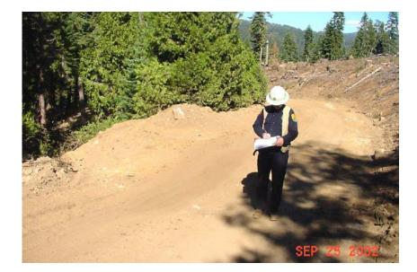
Figure 13. Pete Cafferata, CDF, recording road observations at a rolling dip. Orange box on his right hip is a hip-chain which meters-out string for tracking distances of specific road-related features along a 1000-foot sample segment.
