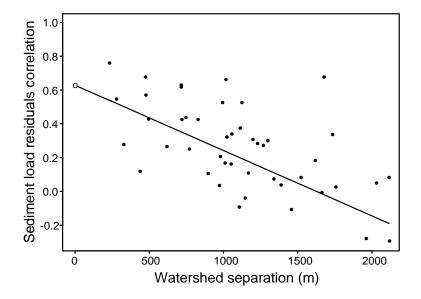
Figure 24. Relation between sediment residuals correlation and distance between watershed centroids. Residuals are from maximum likelihood fit to sediment model {(24),(17),(18)}. Curve depicts equation (17), with estimated parameters  $\hat{\theta}_1$  and  $\hat{\theta}_2$ .
