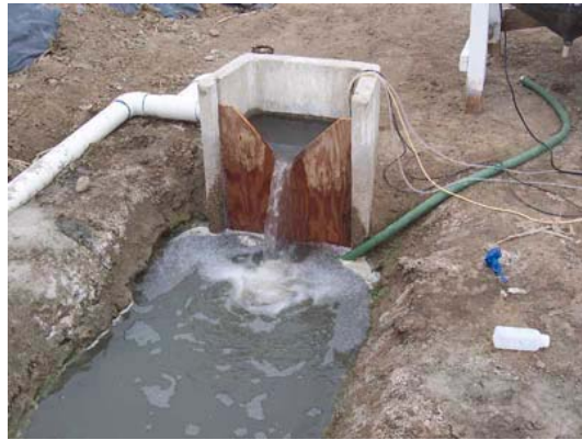
Injection tubes dripping PAM and alum solutions into the inflow monk box and a view from the drain monk box.
