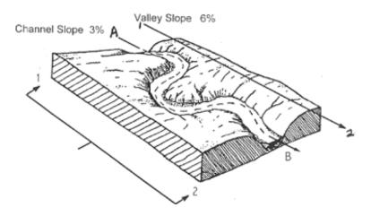
Figure 6-7. Gradient Reduction by Increasing Sinuosity
