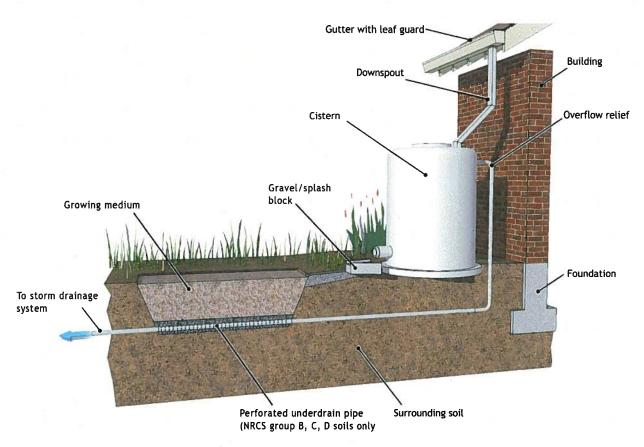
Figure 7. Cistern with Bioretention BMP Example Illustration
