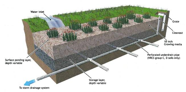
Figure 6. Bioretention BMP Example Illustration
