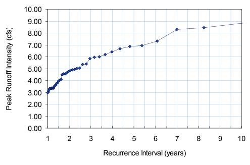
Figure 6-11. Post-Developed (Unmitigated) Flow Frequency Basin A
