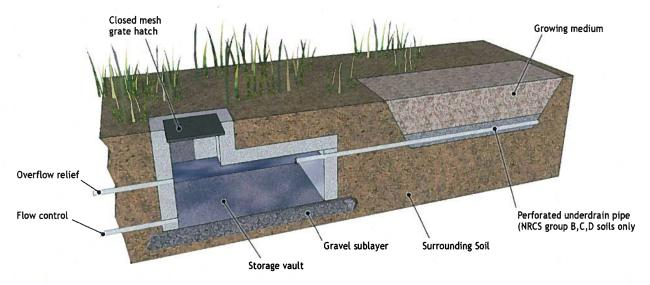
Figure 8. Bioretention with Vault BMP Example Illustration
