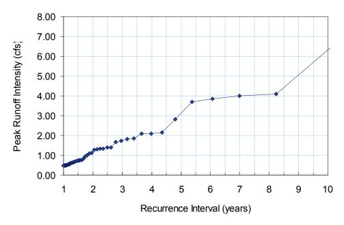
Figure 6-10. Pre-Developed Flow Frequency Basin A
