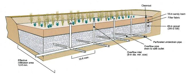
Figure 3. Cross-Section View of Bioretention BMP, Group C/D Soil Configuration
