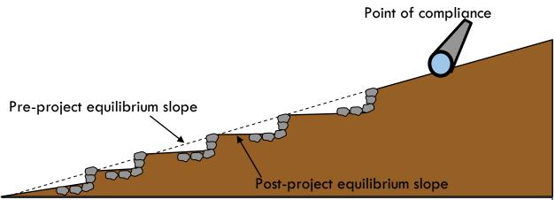
Figure 6-6. Gradient Reduction Using Step-Pool Structures
