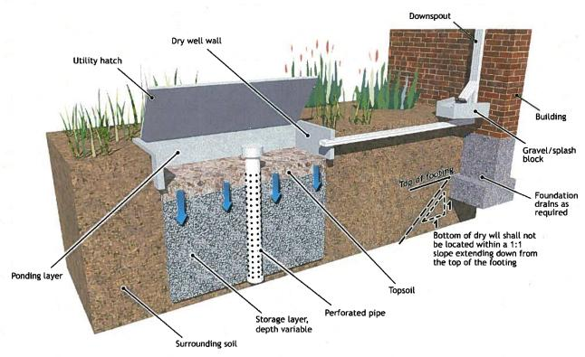
Figure 10. Dry Well BMP Example Illustration
