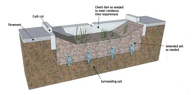
Figure 11. Vegetated Bioswale BMP Example Illustration
