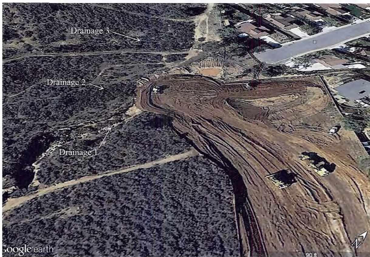
Figure 6. December 2014 Google Earth photo of initiation of grading activity for off-site road knuckle.
