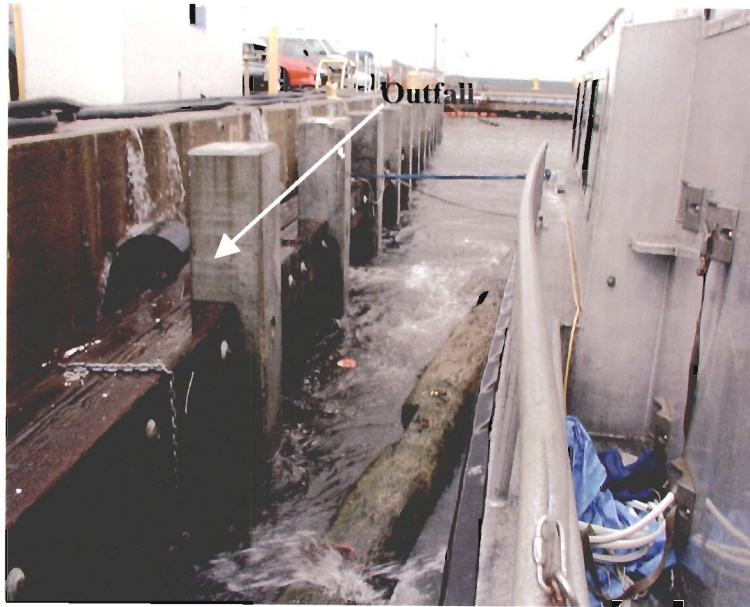
Figure 57. RV ECOS tied up along Naval Station San Diego quay wall outside outfall 14 during the special floating laboratory bioassay conducted in October 2004. The sensors and pump intake were ~ 15 feet away from the outfall. Note sheet runoff over quay wall.
