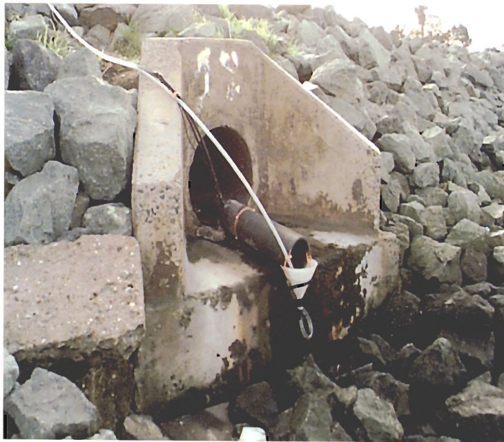
Figure 16. Sampling setup at Naval Amphibious Base Coronado outfall 18. Storm water was sampled as it flowed through the funnel setup, which maintained a continuous 0.5-L volume using the attached siphon tube.
