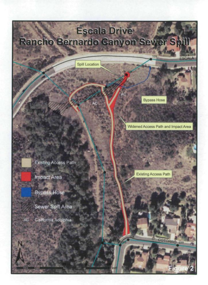
along with a restoration plan. It is anticipated that most of the habitat impacted by the spill will re-establish on its own. The area around manhole 108 which was eroded by the spill will need to be repaired by filling in the ruts, restoring the soil surface, installing erosion control, hydroseeding, and/or planting. The only areas that would be proposed for planting and/or seeding are the areas where the soil surface was disturbed.
