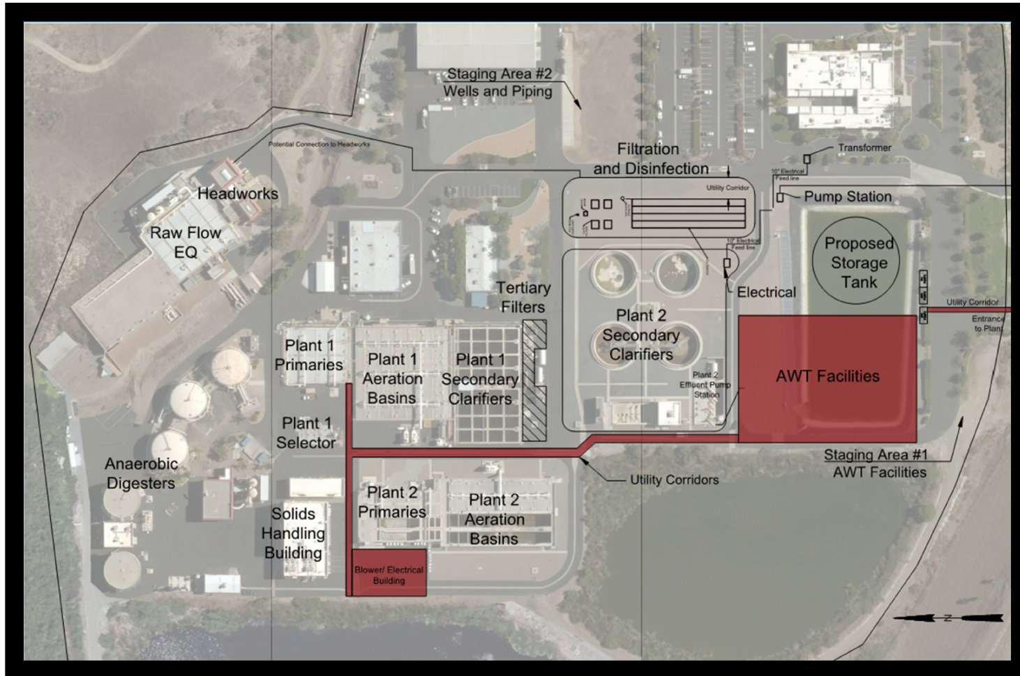
FIGURE B-2 SAN LUIS REY WATER RECLAMATION FACILITY SITE PLAN WITH PROPOSED ADVANCED WATER PURIFICATION FACILITY
