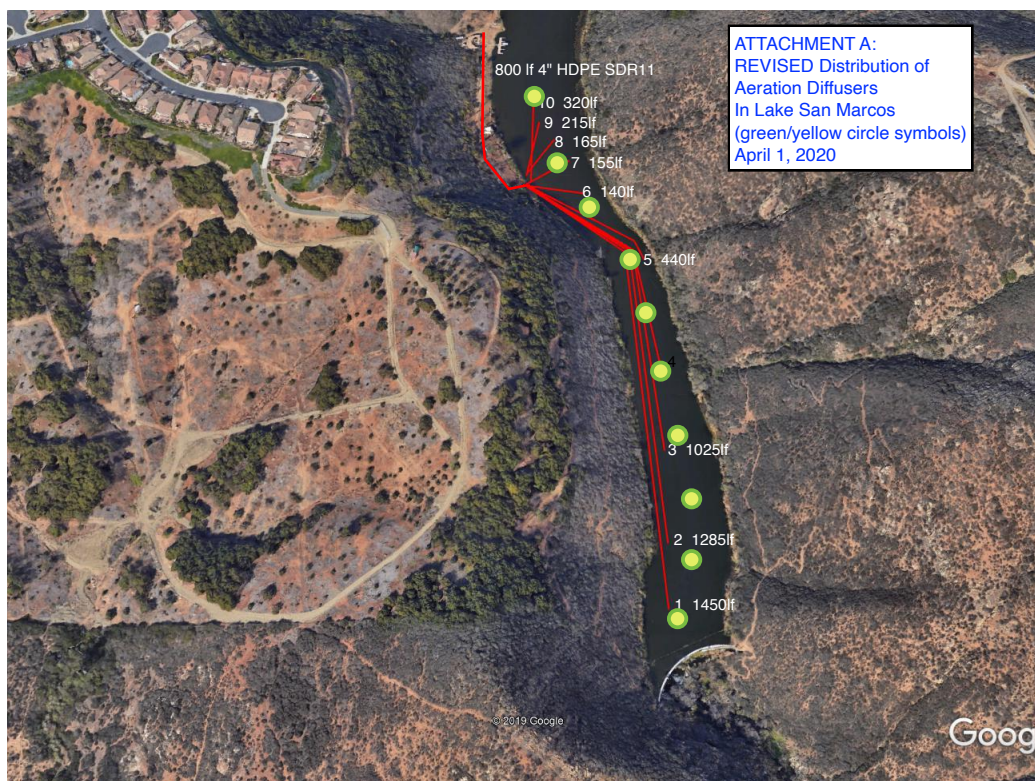
Figure 1. Aeration Diffuser Location
