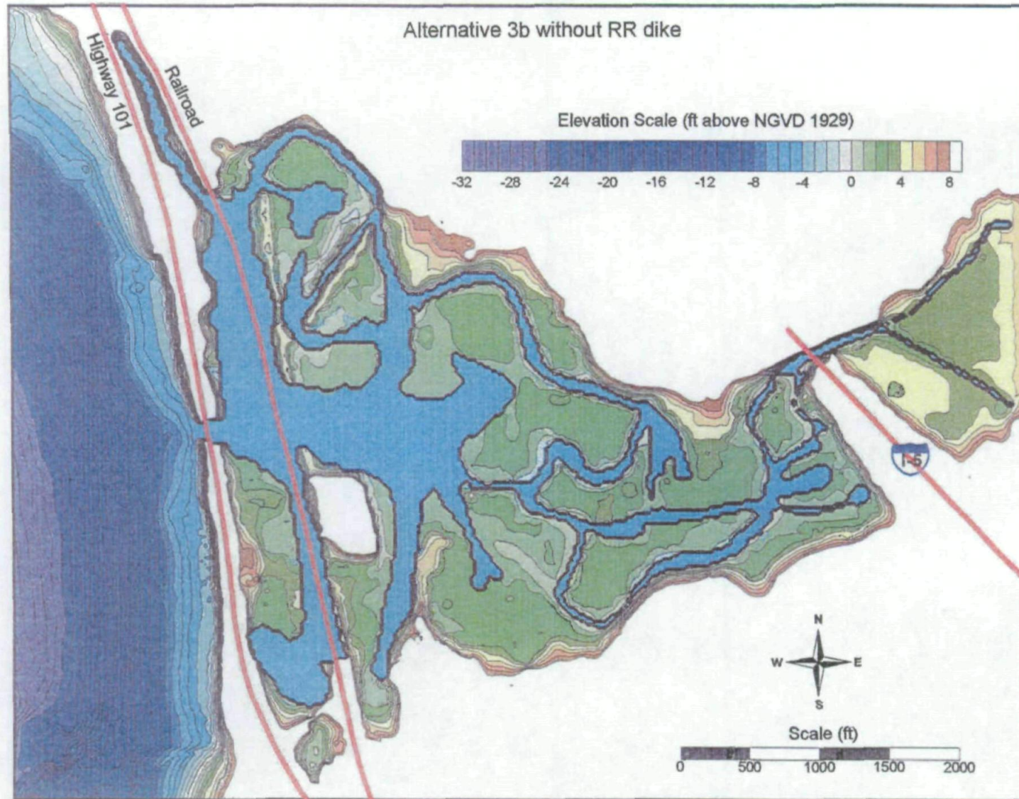
Figure B-6. Lagoon bathymetry after dredging for lagoon inlet Alternative 3 with railroad berm removed.
