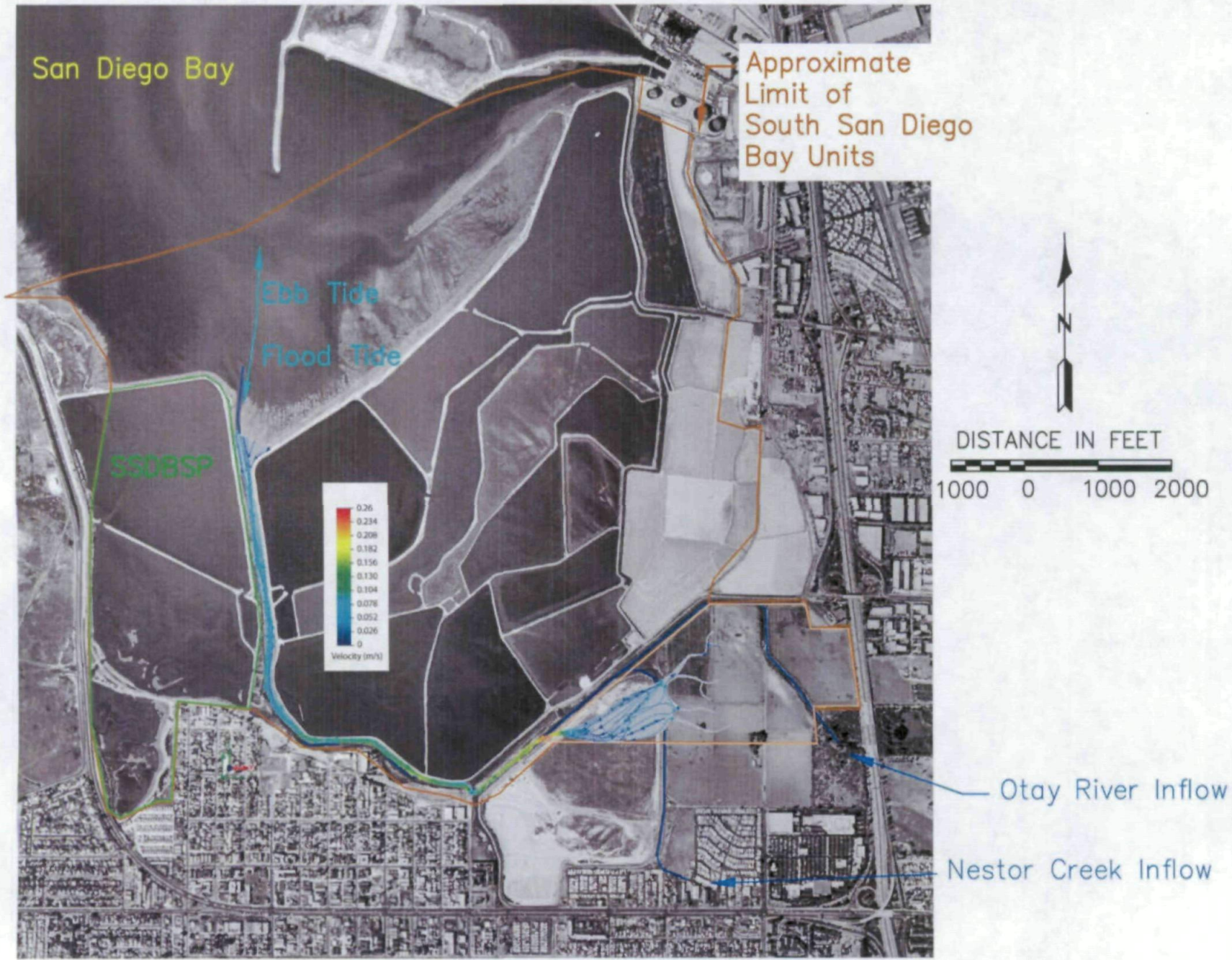
Figure 5b. Far field of hydrodynamic simulation of mean ebb tide flow out of proposed Otay River tidal basin.
