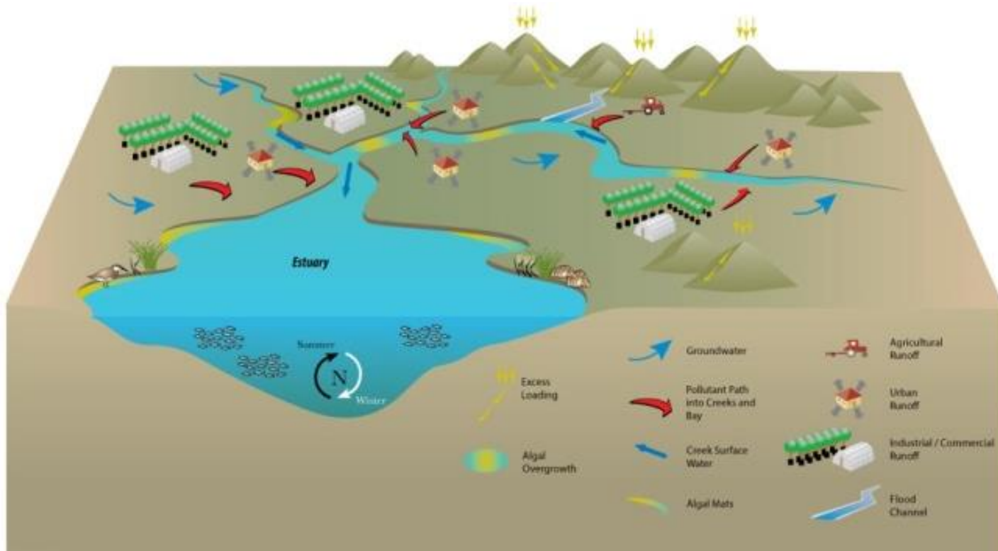
Figure 2.5.4: A graphical conceptual model of nutrient dynamics in a generalized estuarine system. Nutrients derive from multiple sources, both natural and anthropogenic, spread across the watershed. Atmospheric deposition can exceed the carrying capacity of upland soils, leading to nutrient loading to streams during storm events. Nutrient loadings are higher in wet weather and they can be stored in and move through sediments, groundwater, and riparian and aquatic plants on different timescales. Because of these reservoirs, nutrients can require a lengthy period to move through the system and their impacts can continue long after inputs have been shut off. Note: Nutrients enter coastal systems through a variety of sources and pathways.
