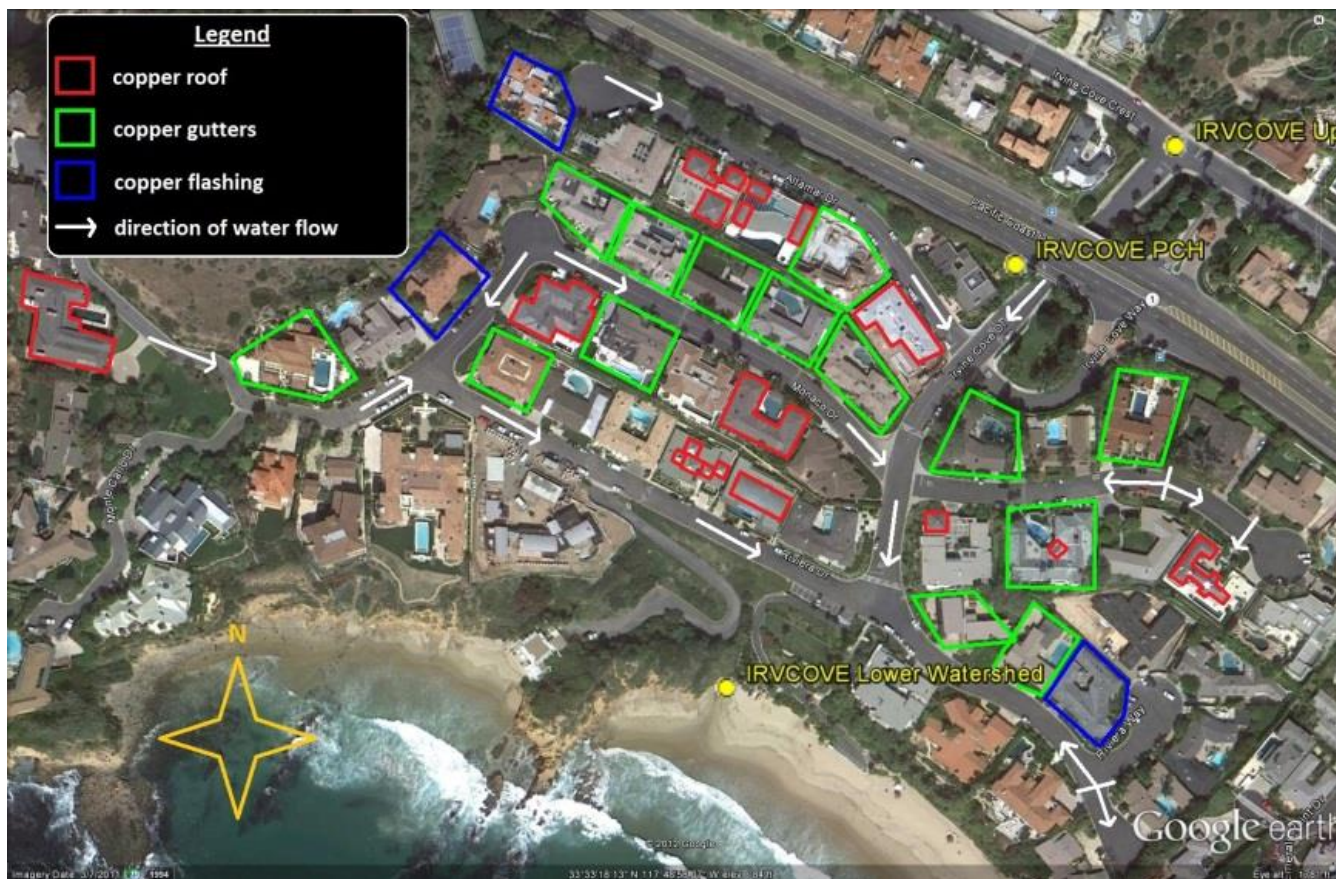
Figure 2.6.4: Aerial photograph of a portion of the Irvine Cove drainage area identifying various types of structural architectural copper uses.
