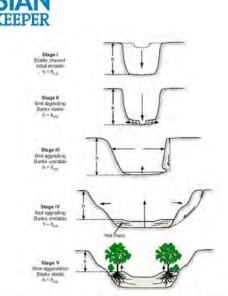
Figure 1: Illustration demonstrating how an incised river channel will naturally erode embankments until it has found its natural course and velocity. Only at that point will banks stabilize.
