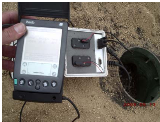
Photo 5. Data loggers attached to a Palm ® device
