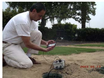
Photo 2. Data from the Aquaflex ® sensors being uploaded
