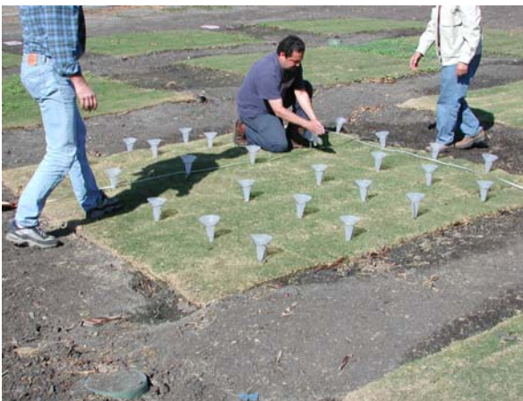
Photo 7. Setting up catch cans to measure the precipitation rate
