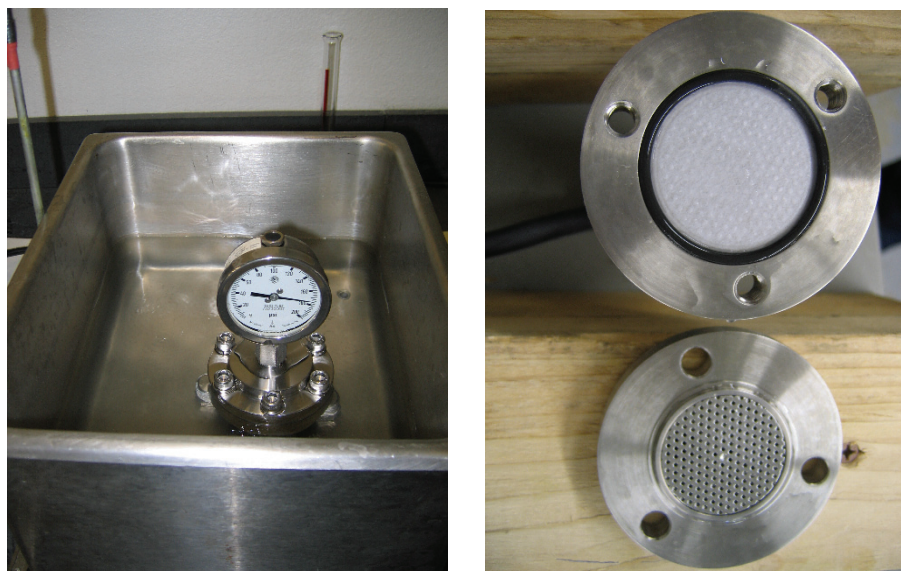
(a) Top view of the DCMO device with a pressure gauge. (b) Tested solutions are injected into the fluid chamber, and the resulting pressure is measured at the pressure port.
