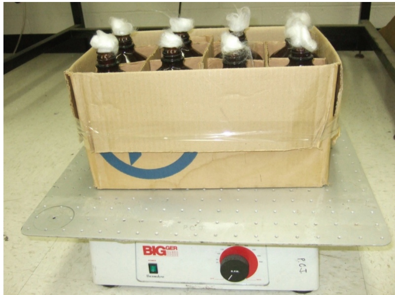
Figure 3.7. BOD reactor with biologically active sand.
