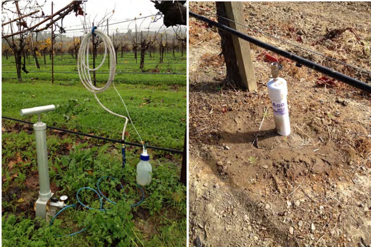
Equipment used for soil pore water sampling. Left, suction lysimeter used to sample at 2 foot and 4 foot depths. Right, suction lysimeter used by AGQ to sample at 20, 40 and 60 centimeters (approx.. 8, 16, and 24 inches).
