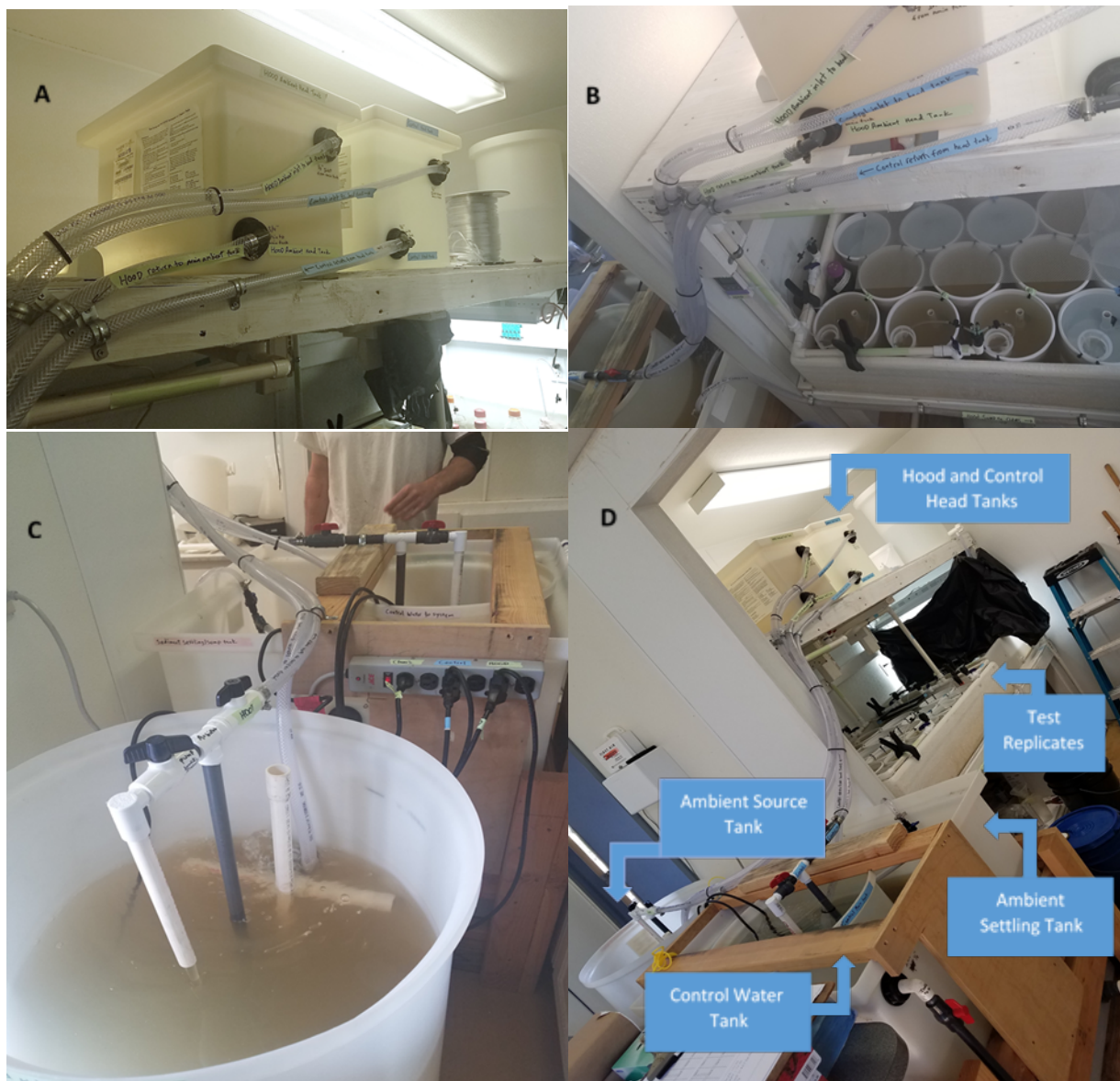
FIGURE 3: EX-SITU IMPROVEMENTS, INCLUDING: A) HEAD TANKS ADDED TO THE EX-SITU SYSTEM; B) RETURN FLOW TO THE CONTROL WATER TANK; C) RETURN TO THE AMBIENT SOURCE TANK; D) OVERVIEW OF THE EX-SITU SYSTEM WITH ADDITIONAL HEAD TANKS INSTALLED.
