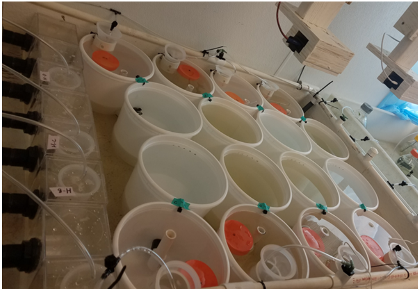
FIGURE 11: SECONDARY H. AZTECA REPLICATE CAGES (ORANGE CAPS) WERE INCLUDED DURING THE SECOND EXPOSURE PERIOD AND PLACED IN THE SETTLING TANK PORTION OF THE RAINBOW TROUT REPLICATES.
