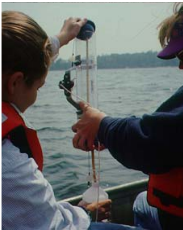
Figure 4. The Van Dorn sampler is effective for discrete depth sampling.
