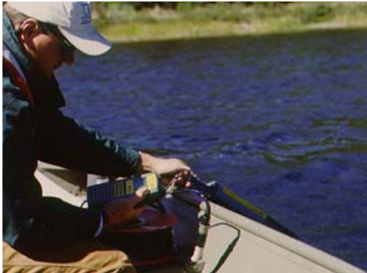
Figure 3. A multiprobe sonde lowered through the water column can analyze several variables simultaneously while being monitored from the lake surface.
