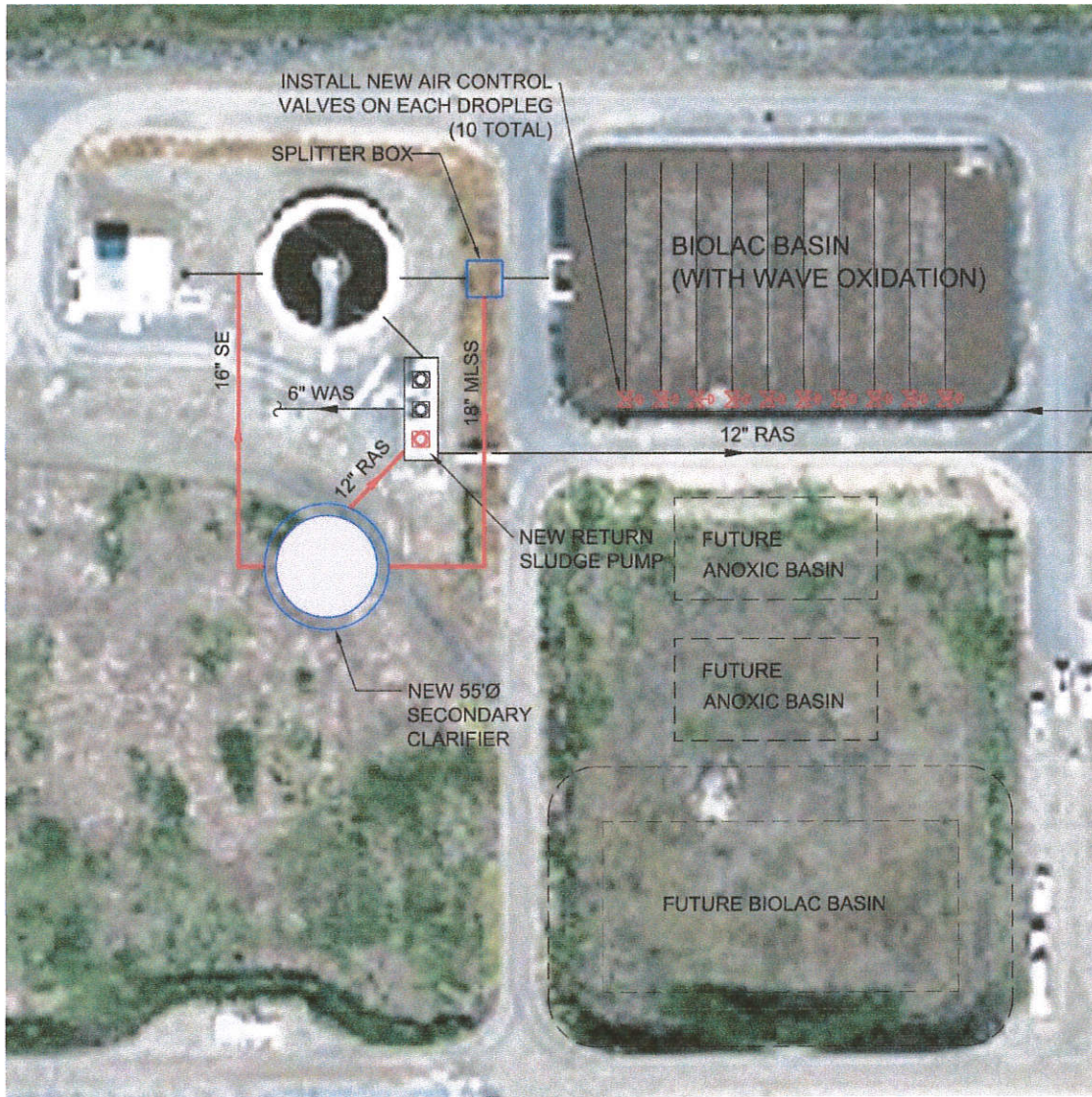
Figure 3 Proposed WWTP Improvements for Denitrification
