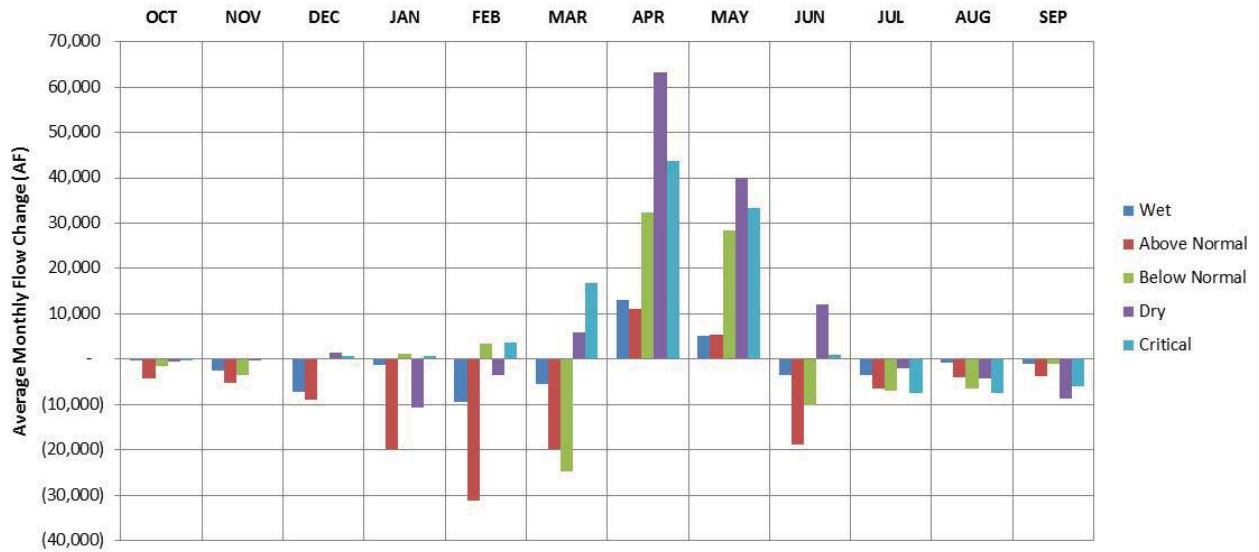
Figure 7: Average Monthly Flow Change (AF) at Smartsville Gage from Baseline Conditions for the 40 Percent Unimpaired Flow Scenario by Year Type
