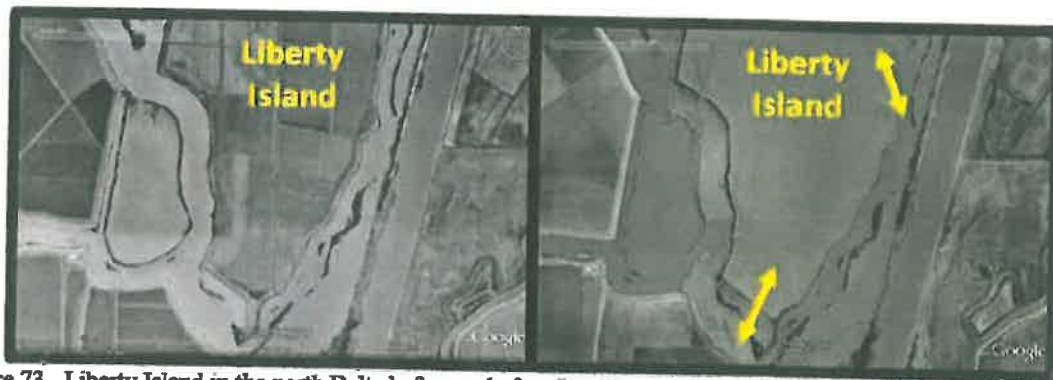
Figure 73. Liberty Island in the north Delta before and after flooding showing locations of narrow breaches in the levee.
