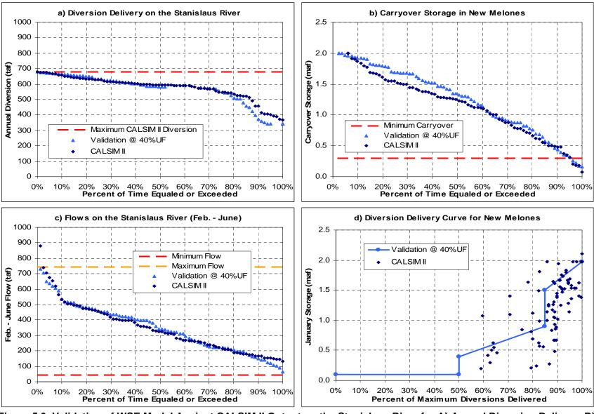
Figure 5.3. Validation of WSE Model Against CALSIM II Output on the Stanislaus River for A) Annual Diversion Delivery, B) End-of-September Storage, C) Flow at CALSIM II Node 528, D) Diversion Delivery Rule Curve Based on January Storage Level
