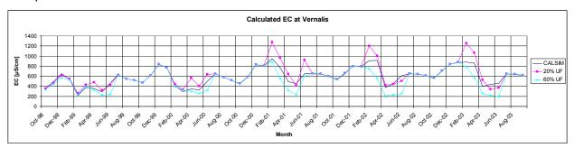
Figure 4.6. Calculated EC at Vernalis for the 40% and 60% Unimpaired Flow Example Compared to CALSIM II Results for Water Years 1994–2003
