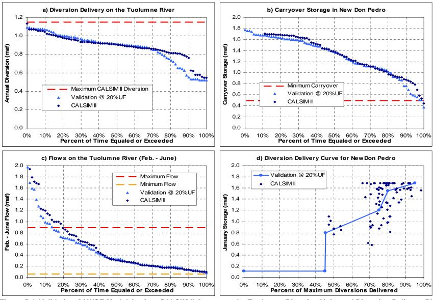
Figure 5.4. Validation Of WSE Model Against CALSIM II Output on the Tuolumne River for A) Annual Diversion Delivery, B) End-of-September Storage, C) Flow at CALSIM II Node 528, D) Diversion Delivery Rule Curve Based on January Storage Level
