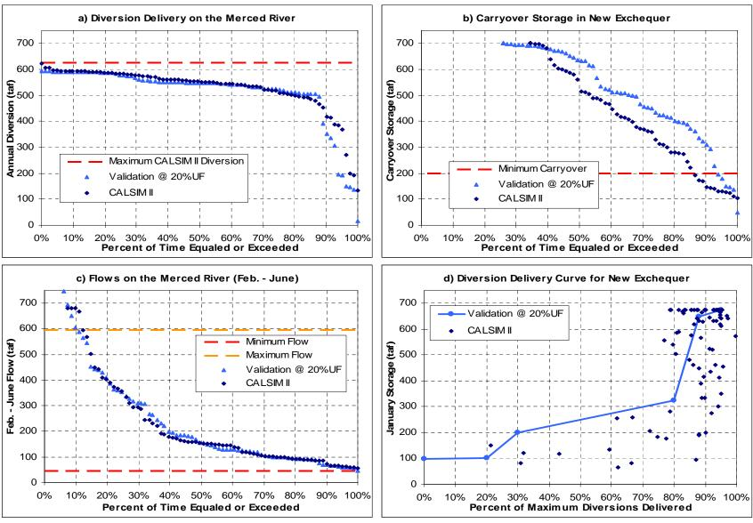
Figure 5.5. Validation of WSE Model Against CALSIM II Output on the Merced River for A) Annual Diversion Delivery, B) End-of-September Storage, C) Flow at CALSIM II Node 528, D) Diversion Delivery Rule Curve Based on January Storage Level
