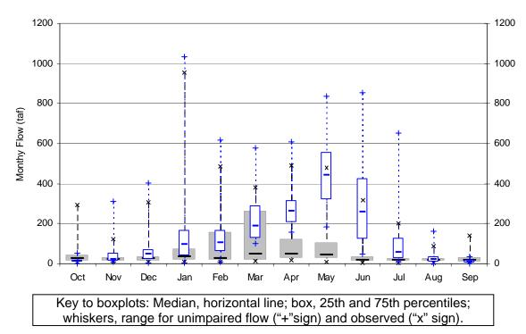
Figure 2.11. Monthly Unimpaired Flow (Open Bars) and Observed Flow (Filled Bars) in the Tuolumne River from 1984 to 2009
