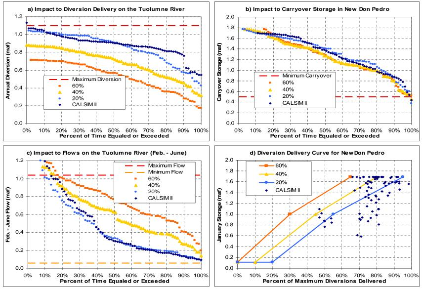
Figure 5.7. Results of Impacts for Illustrative Flow Objective Alternatives of 20%, 40% and 60% of Unimpaired Flow on the Tuolumne River
