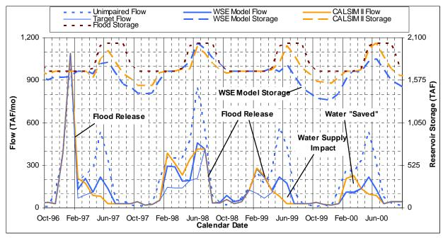
Figure 5.2. Monthly Unimpaired Flow and 40% of Unimpaired Flow Objective Alternative Compared to CALSIM II Flow on the Tuolumne River at CALSIM II Node C545
